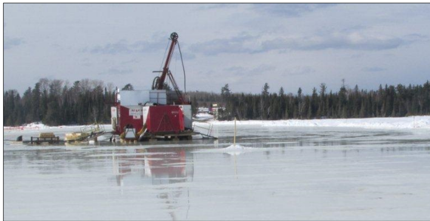
Photo 13: Diamond-drill rig on ice during the winter.
