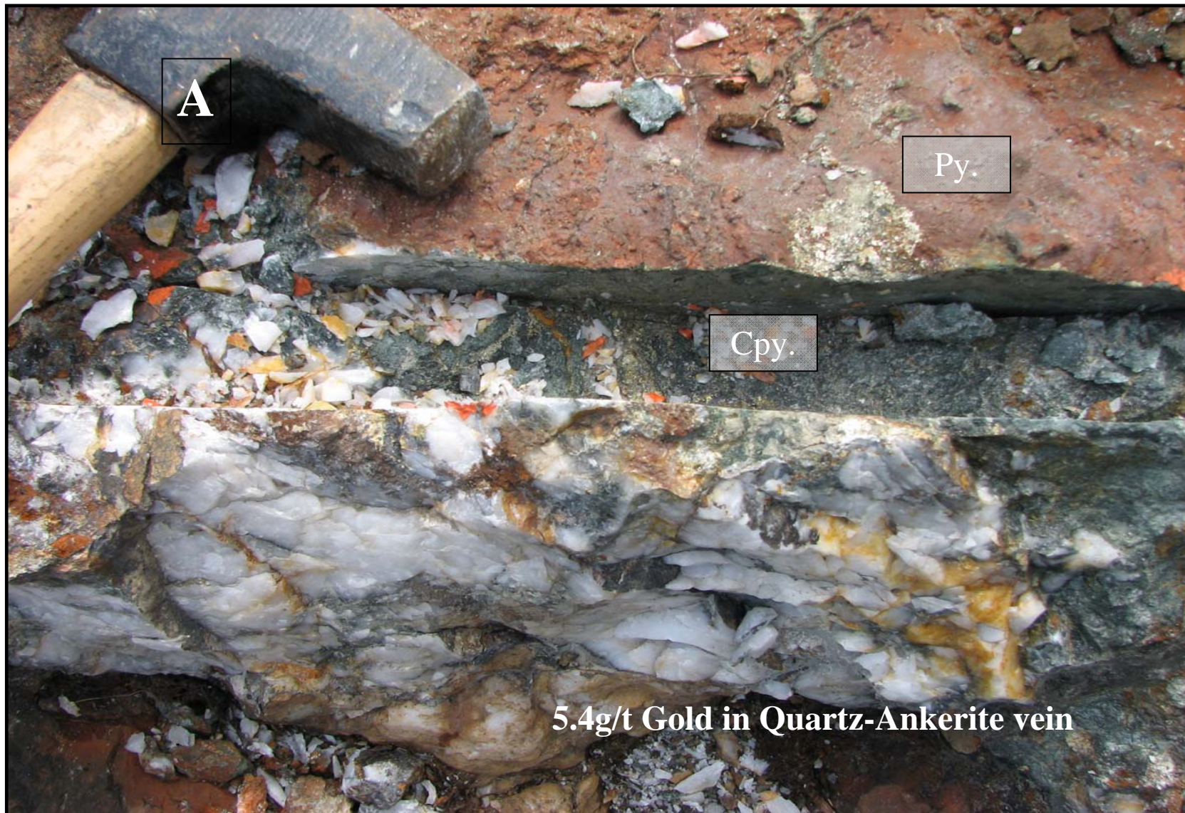
Figure 4.2.1.3: Semi-massive Sulphides Associated with Quartz-Ankerite Veins in Mafic Volcanics (Location A)
