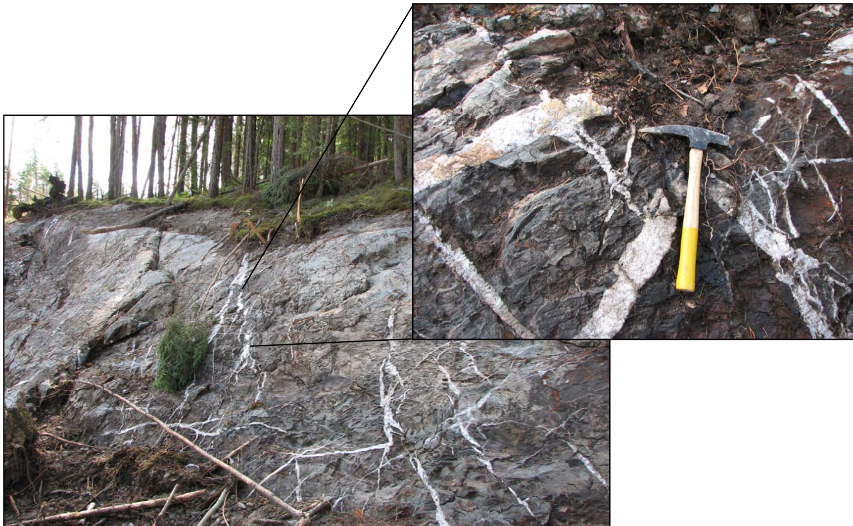
Figure 4.2.9.4: Quartz-Ankerite Veins in Mafic Volcanics with Detail Insert (Location C)
