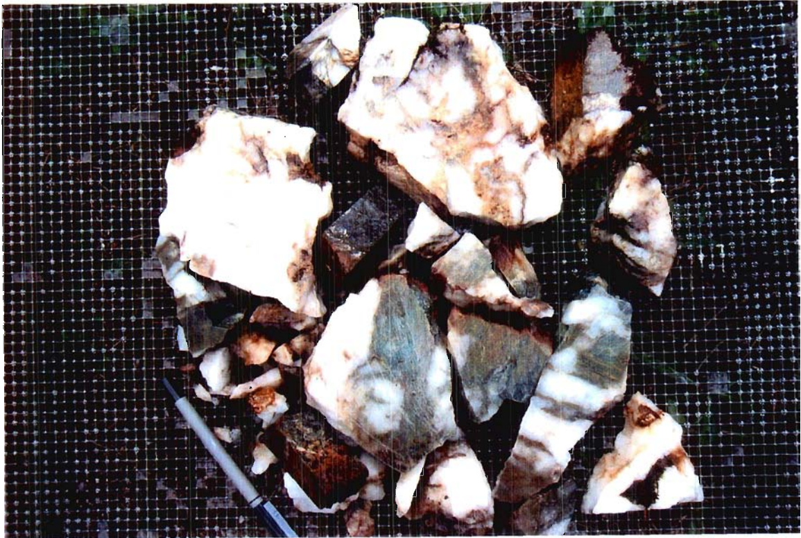
Photo 5. Quartz-ankerite veining in channel sample 2161, site #4. The 45 cm wide quartz-ankerite vein trends at 52°, and cuts highly carbonatized ultramafic flows. The vein displays well-developed vein parallel crack-seal structures. Wallrock inclusions and margins to the vein are “green carbonate” (weakly-moderately fuchsitic).
