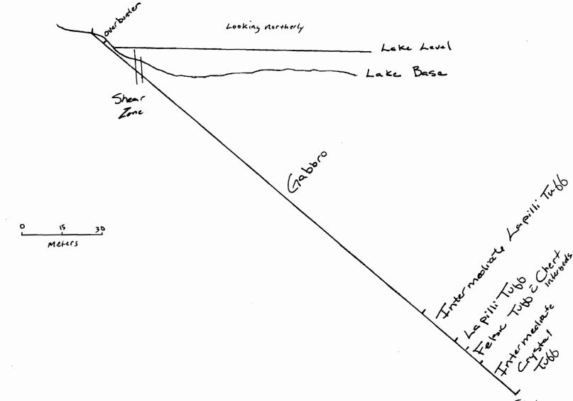
Property:Cedartree Lake Claim No: 1239485 Easting:93 <sup>0</sup> 51.26 W Northing:49 <sup>0</sup> 18.97 N Grid East: 1910 E Grid North: 1019 N Collar Elevation: 336m Core Size: NQ DIAMOND DRILL LOG - SummaryDip:- 40 °Azimuth103 °Depth:206.5 mDown Hole Survey: -38 ° @ 205.4m (acid)
