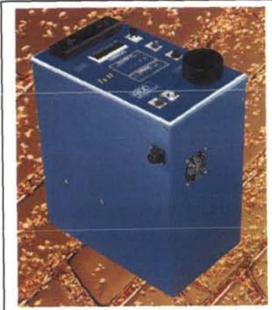
This backpackable 1400 W induced polarization (I.P.) transmitter works from a standard 120 V source and is well adapted to rocky environments where a high output voltage of up to 2 000 V is needed. Moreover, in highly conductive overburden, at 150 V, the highly efficient 1400 W transmitter is able to send a current of up to 10 amperes. By using this I.P. transmitter, you obtain fast and high-quality I.P. surveys in all possible field conditions.
