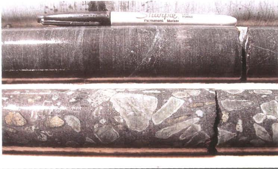
Photo 1: Ultramafic xenoliths surrounded by whitish coloured reaction rims within a lamprophyre (melnoite) dyke.
