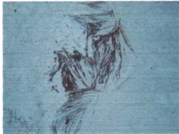
Figure 15. Left: BSE-image of chalcopyrite grain weathering to malachite (top of grain, medium grey) and hematite along fractures (top right of grain); set in hematitized quartz. Calcite occurs in association with the chalcopyrite grains on the bottom of the image. Right: Photomicrograph of acicular and fine-grained hematite in quartz, causing a bright red coloration. The field of view is 2.5 mm.
