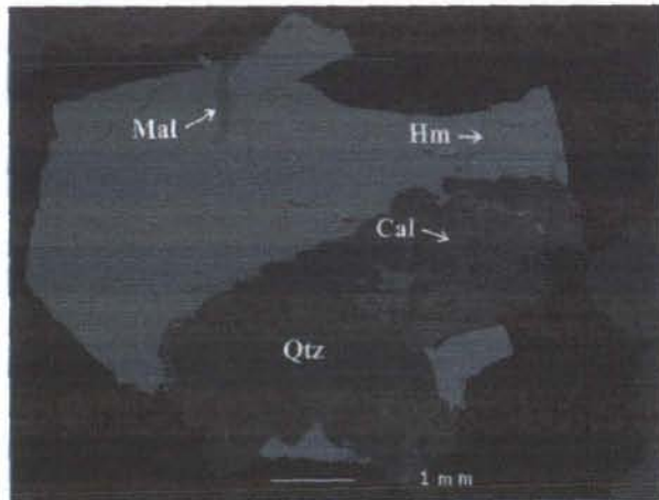
Figure 15. Left: BSE-image of chalcopyrite grain weathering to malachite (top of grain, medium grey) and hematite along fractures (top right of grain); set in hematitized quartz. Calcite occurs in association with the chalcopyrite grains on the bottom of the image. Right: Photomicrograph of acicular and fine-grained hematite in quartz, causing a bright red coloration. The field of view is 2.5 mm.
