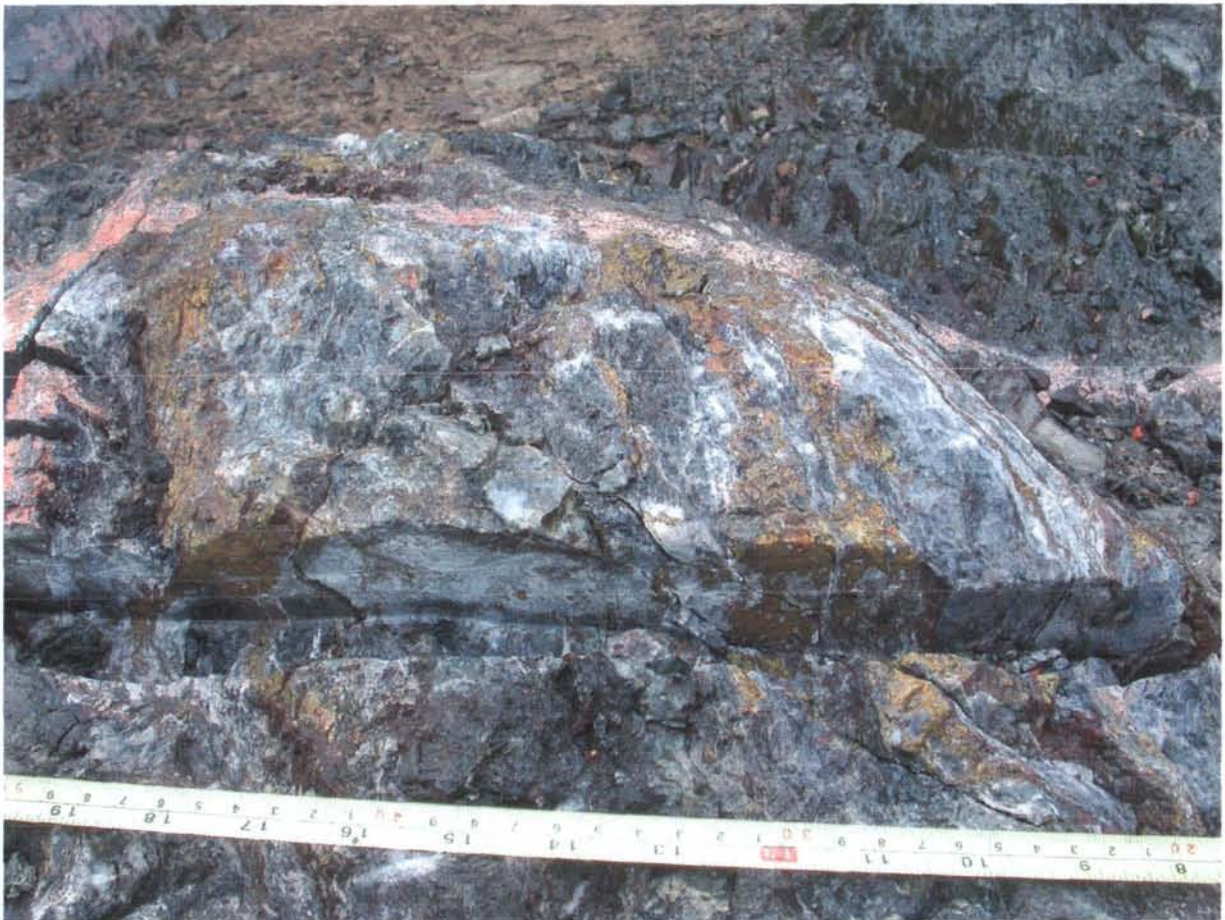
Figure 9: Cu-Au-Ag-Co Quartz-Carbonate vein, 10 m east of the Merico Shaft; assayed 5.99 g/t Au, 8.6 g/t Ag, 6.33% Cu, 0.27% Co over 5 m.
