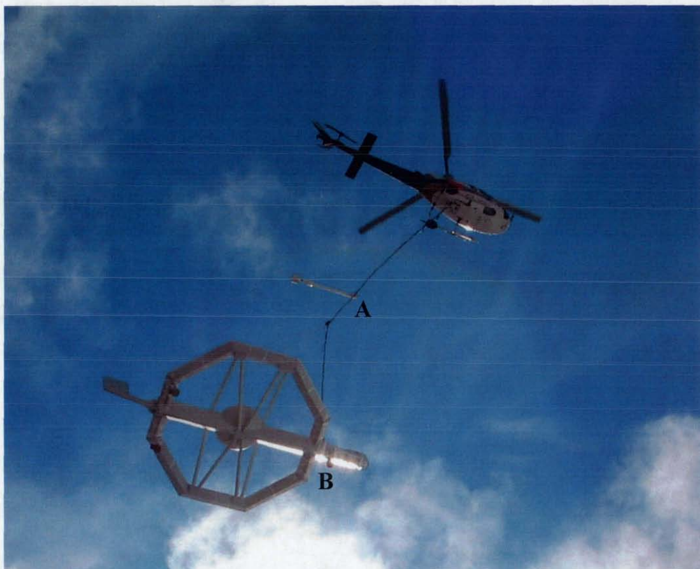
Figure 3. The magnetometer bird (A) and AeroTEM II EM bird (B)
