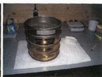
Typical sieve arrangement
