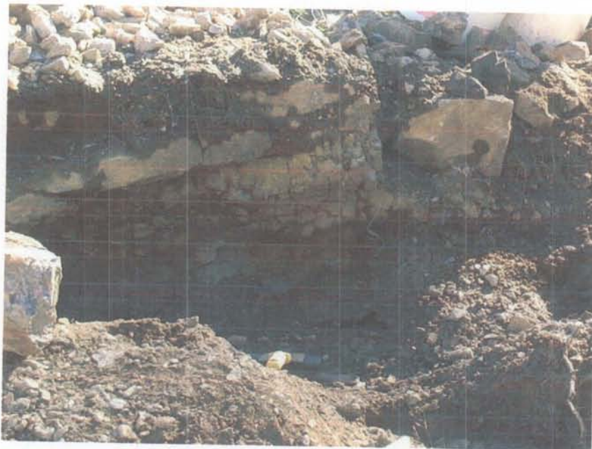
Photo 7: Excavation of second vug. Top of photo shows granite hanging wall with 10cm amethyst vein attached.
