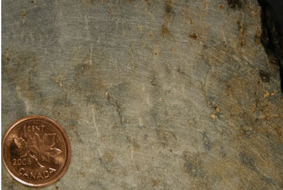
Figure 13. Slabbed vein from the Bonanza trench showing visible gold.
