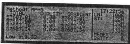
Close-up of the ENVI-MAG screen showing data presented after each reading
