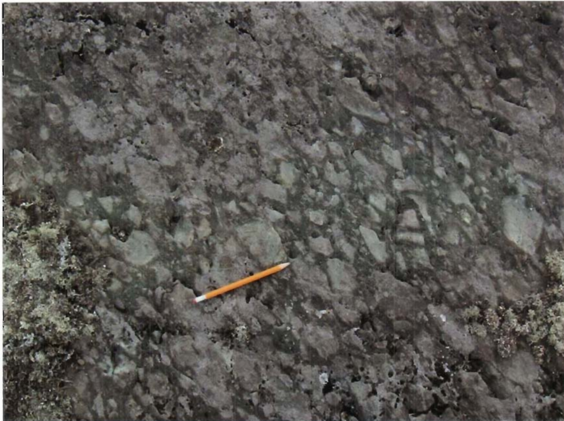
Fig. 4. Mafic, broken-pillow breccia in lower mafic metavolcanic sequence (438600E, 5419760N). Partial pillow selvages, where present, are dark grey.
