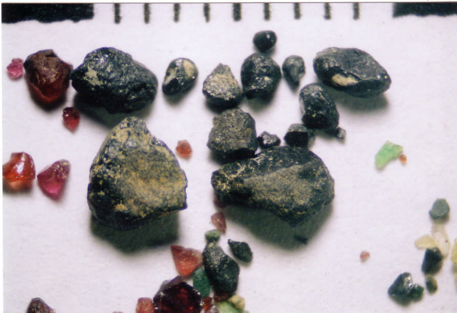
Figure 19. : Picroilmenite and chromite showing excellent preservation of resorption features on grain surfaces. Sample 2E, 2A Site Top Scale 1 cm
