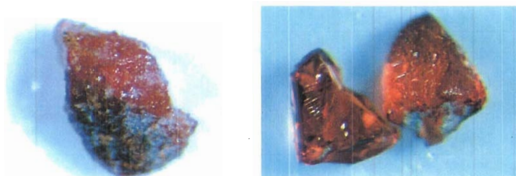
Photo 2 – Eclogitic garnet from 32170 (left) as rock fragment from eclogitic nodule and from 40290 (right) with intensive orange color and resorption features.
