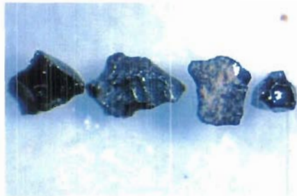
Photo 8 – Four morphologically different picroilmenites from 40439: fractured, matte, “bumpy” with yellow coating and polygranular.
