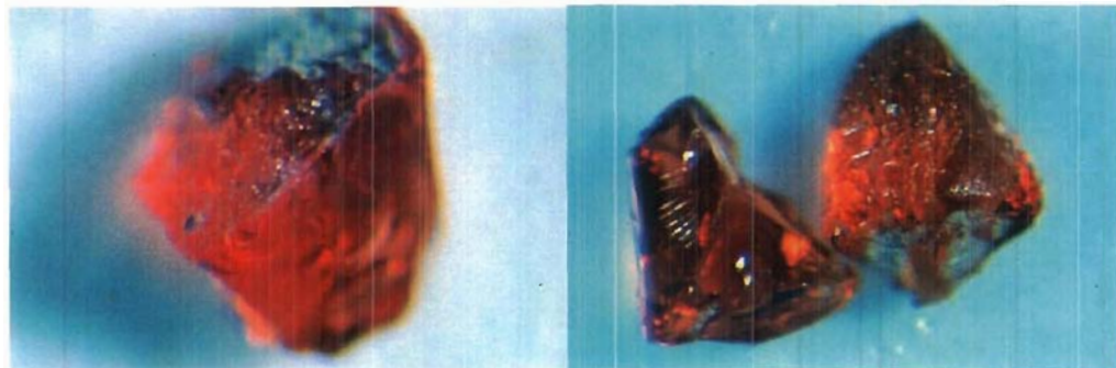
Photo 6 - Slightly abraded fractured EG with patch of surface layer and slightly abraded fractured edges (40164 left and 40290 right)
