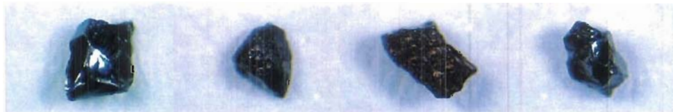
Photo 13 – Sample 40165 and four picroilmenites representative for the four morphological groups: fractured, matte, “bumpy” and polygranular (from left to right).
