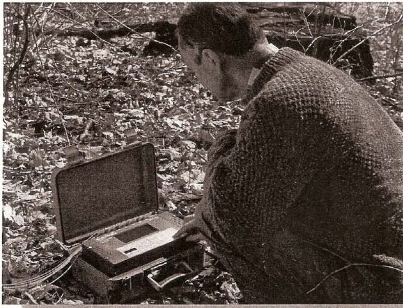
The IPR-12 Receiver measures eight dipoles simultaneously then records measured and calculated parameters in memory.
