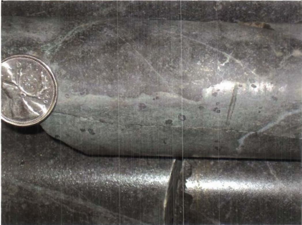
Fig. 10. Chilled, irregular margin of a paler-grey, quartz-phyric, felsic dike intruded into a darker-grey, more altered, quartz- + plagioclase-phyric, felsic dike; the younger dike is subparallel to the core axis. The younger dike truncates narrow calcite veins in the older dike. This contact is in the composite felsic sill that forms the east contact of the Off Lake felsic dike complex. Drill hole OF07-03, 81.5 m; quarter for scale.
