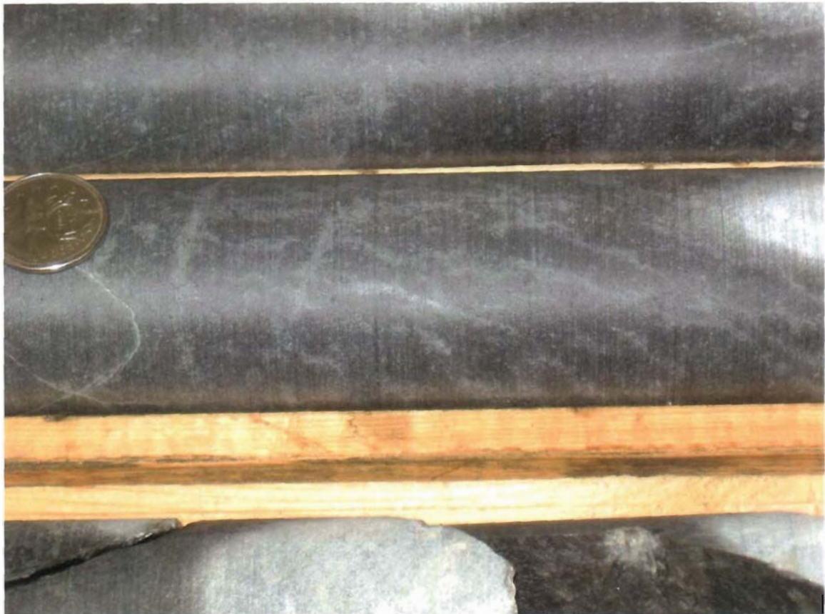
Fig. 15. Flattened, fracture-controlled, bleaching in a quartz-phyric, felsic dike of the composite felsic sill that forms the east contact of the Off Lake felsic dike complex. Drill hole OL07-03, 145 m; quarter for scale.
