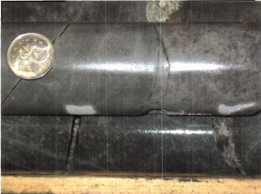
Fig. 11. Contact between a younger, quartz-phyric, felsic dike on left and an older, more altered, quartz-phyric felsic dike on right; contact is marked by a 1-mm-wide, quartz vein or silicified zone. This contact is in the composite felsic sill that forms the east contact of the Off Lake felsic dike complex. Drill hole OL07-03, 96.4 m; quarter for scale.
