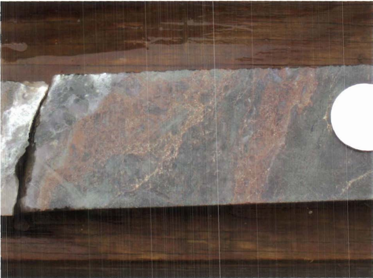
Fig. 32. Semi-concordant zones of sphalerite and pyrite mineralization in foliated and altered metagabbro. Within the red-brown, sphalerite-rich zones, the sphalerite occurs as interconnected networks of fine veinlets, which form about 30% of the zones; minor calcite is associated with the pyrite. On the left, a late quartz vein transects a sphalerite-rich zone. Drill hole OL07-03, 245.0 m; quarter for scale.
