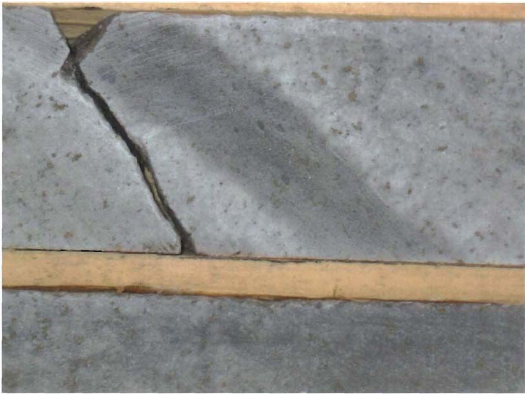
Fig. 13. A 1-cm-wide, dark-grey, quartz-phyric, felsic dikelet intruded into a paler-grey, more altered, quartz-phyric, felsic dike that contains fewer quartz phenocrysts. This is in a mappable, composite felsic sill about 125 m west of the composite felsic sill that defines the east contact of the Off Lake felsic dike complex. Drill hole OF07-02, 165 m.
