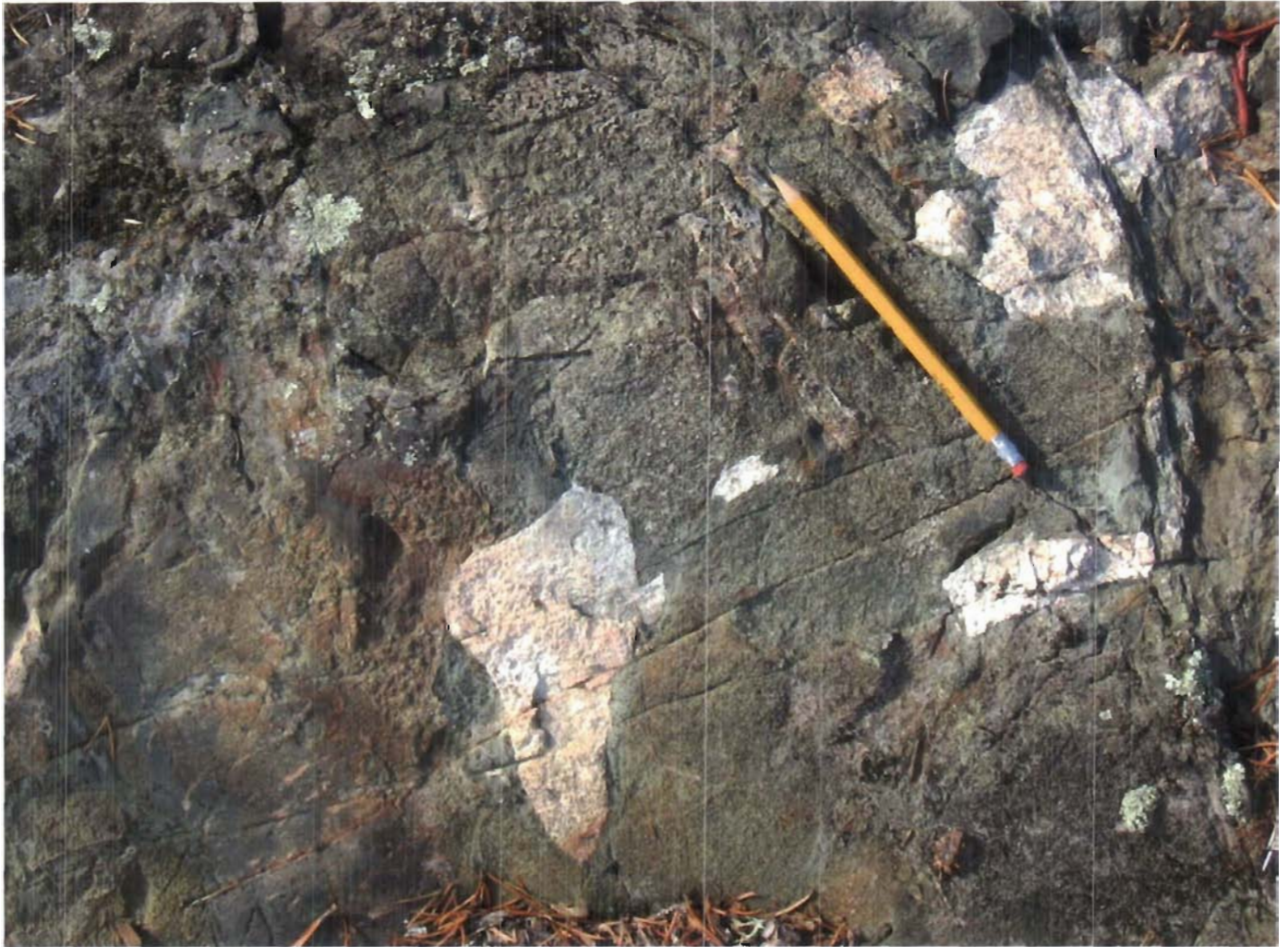
Fig. 4. Polymictic, mafic to felsic volcanic, clast-supported, cobble conglomerate in which mafic clasts dominate (441000E; 5417600N). Mafic clasts are rounded and include both fine-grained volcanic and medium-grained metagabbroic clasts; where fine-grained clasts are in contact, clast boundaries are difficult to discern. Felsic clasts are more angular than mafic clasts. Pencil for scale is about 15 cm long.
