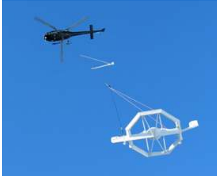
Figure 2: Eurocopter with equipment for Airborne Survey, October 2006.
