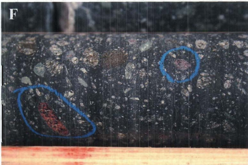
F: Dark grey kimberlite facies with red and purple garnet phenocrysts in hole 07-MF1-01.
