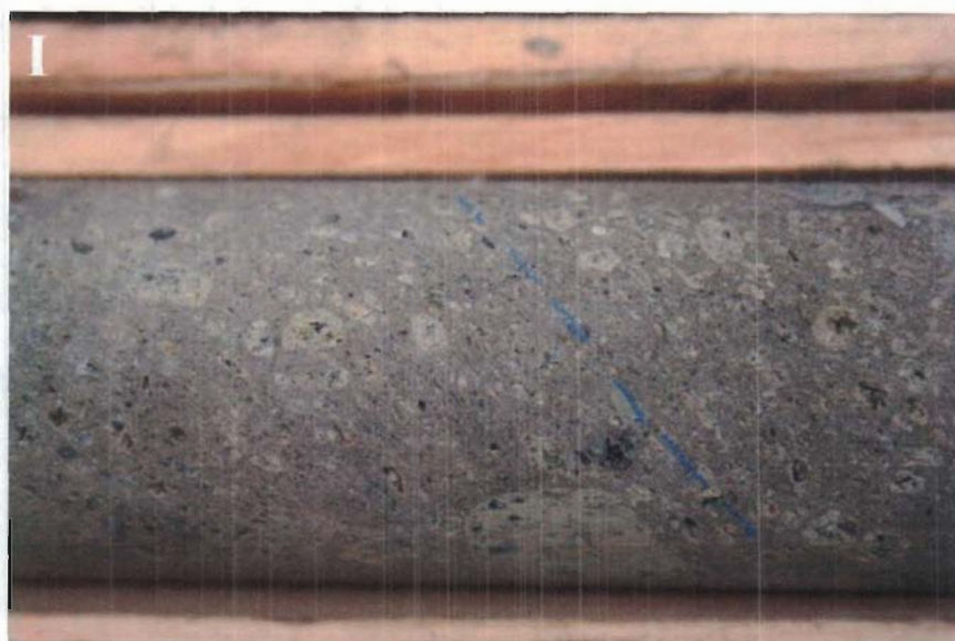
Figure 5 (continued): I: Fine-grained and foliated brown kimberlite facies in hole 07-GF-02-W3
