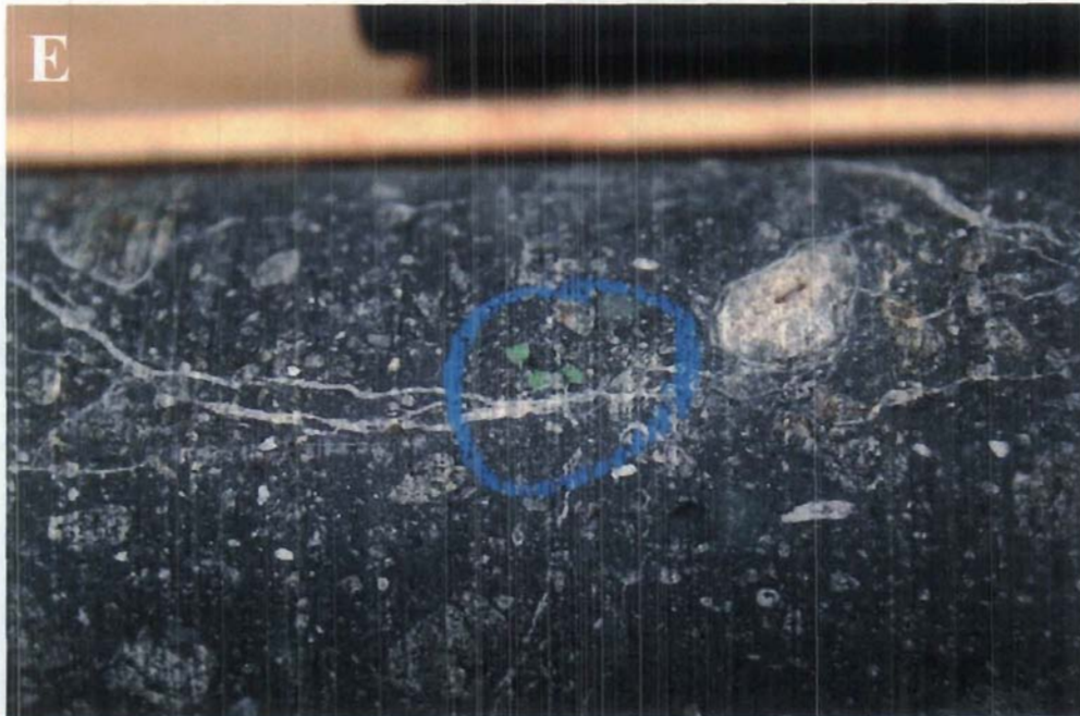
E: Dark grey kimberlite with low phenocryst content. It has Cr diopside phenocryst and olivine – Cr-diopside xenoliths in hole 07-MF1-01.
