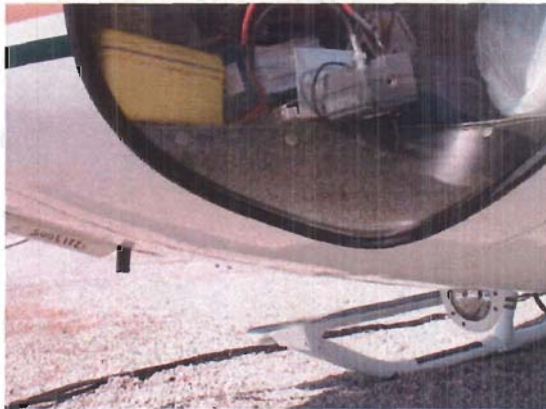
Figure 7. Digital video camera typical mounting location
