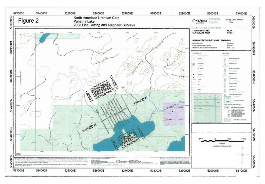
The geophysical program consisted of total field magnetic surveying. The total magnetic field survey, using a GEM GSM-19 magnetometer, totaled 9.79 kilometers with readings collected every **12.5** meters along all lines. A description of the instruments and survey methods can be found in appendix A.
