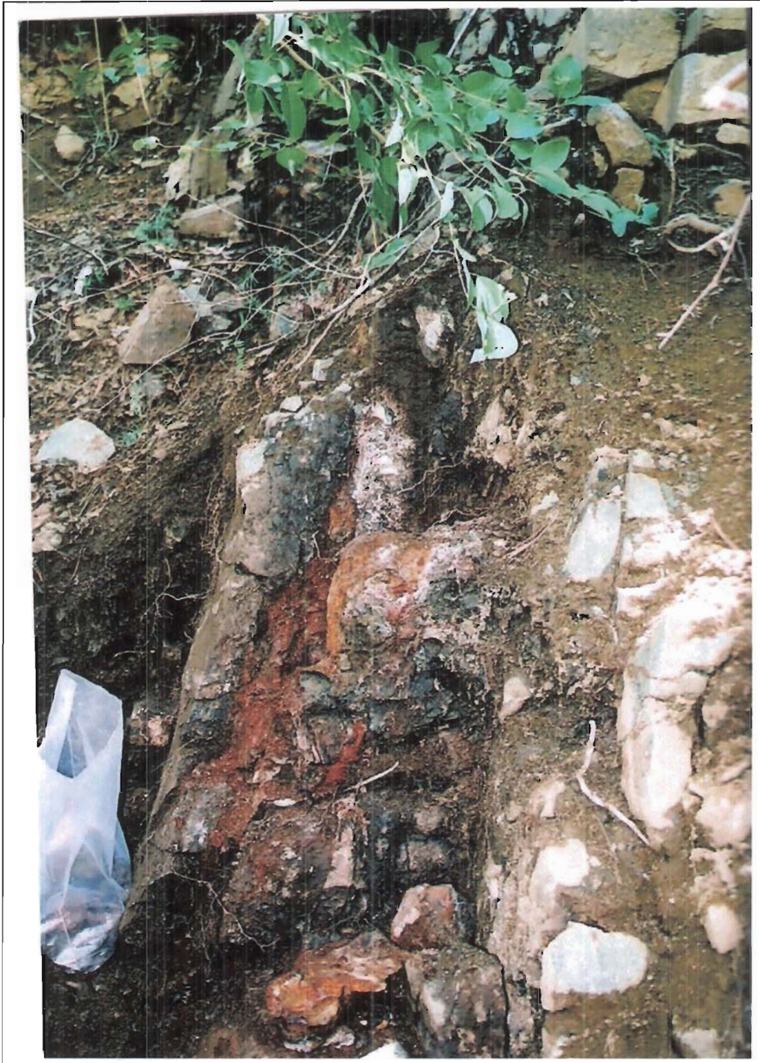
Figure 9. Strong altered 10 cm shear zone along the carbonate vein.
