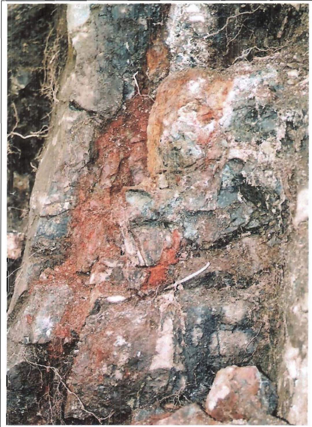
Figure 10. Wall rock alteration of red colored hematite, yellowish limonite (jarosite?), and possibly white kaolin or alunite from metasomatism.
