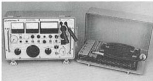
IPC-7 / 2.5kW transmitter console with lid and dummy load.
