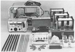
Complete 2.5kW induced polarization system including motor-generator, reels with wire, tool kit, porous pots, simulator circuit, copper sulphate, IPR-8 receiver, dummy load, transmitter, electrodes and clips.
