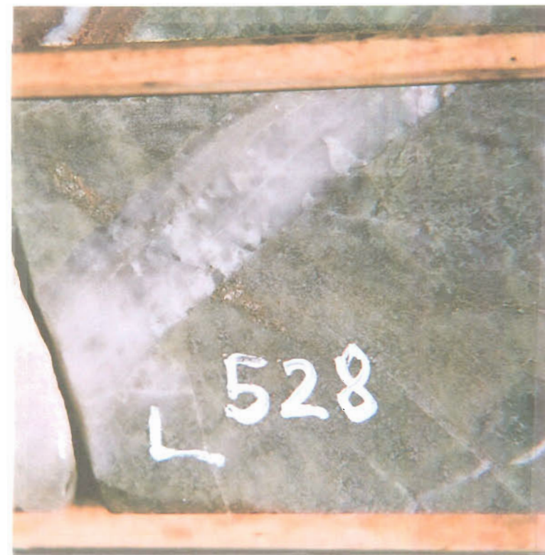
Pyrite veins crosscut by quartz tension gashes (51529, 51528).
