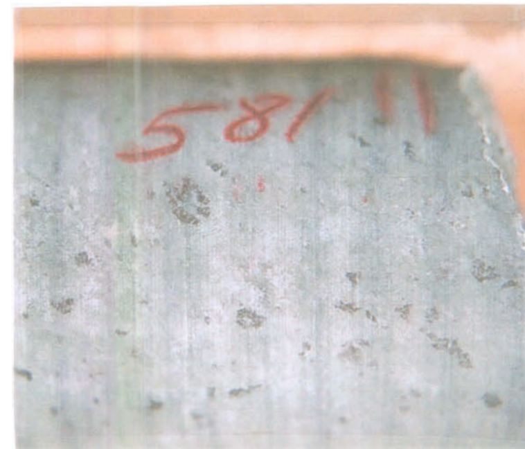
Clusters of octahedrally laminated magnetite-ilmenite in gabbro.
