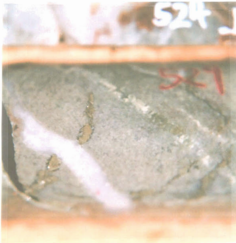
Pyrite veins crosscut by quartz tension gashes (51529, 51528).
