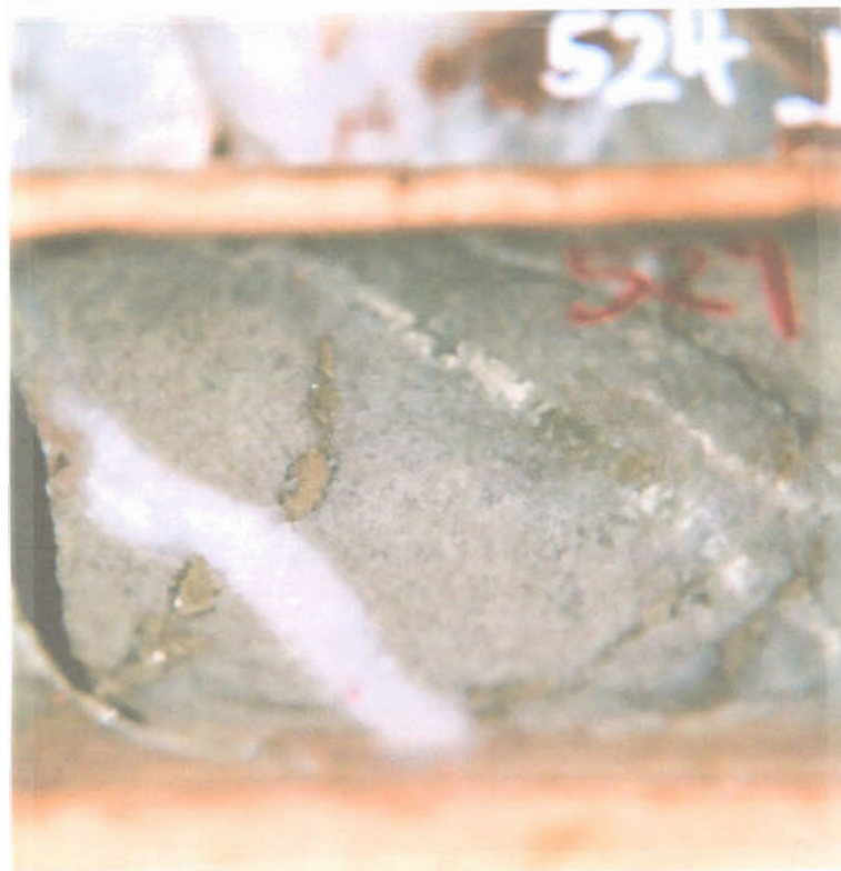
Pyrite veins crosscut by quartz tension gashes (51529, 51528).
