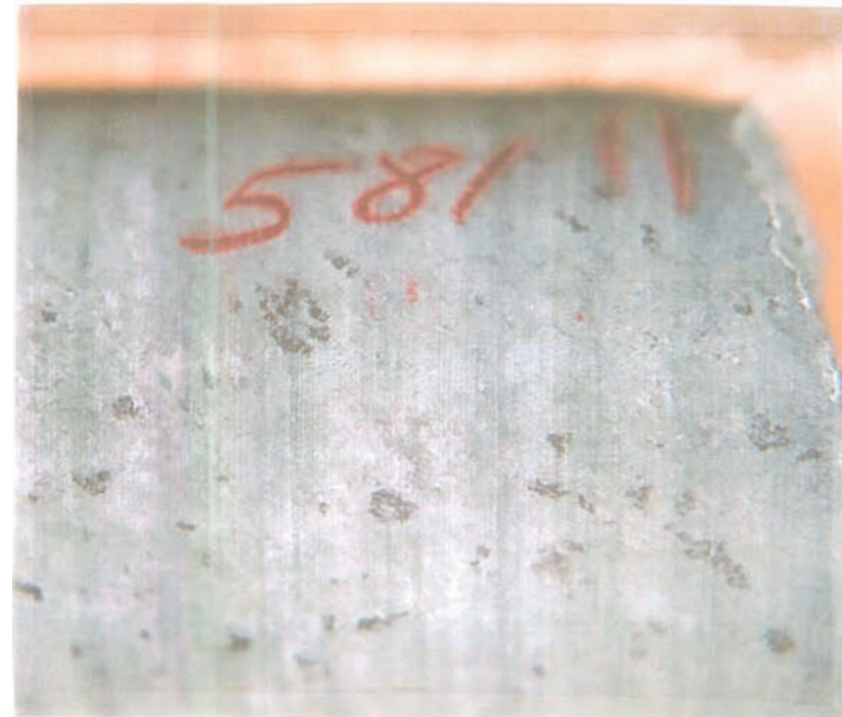
Clusters of octahedrally laminated magnetite-ilmenite in gabbro.
