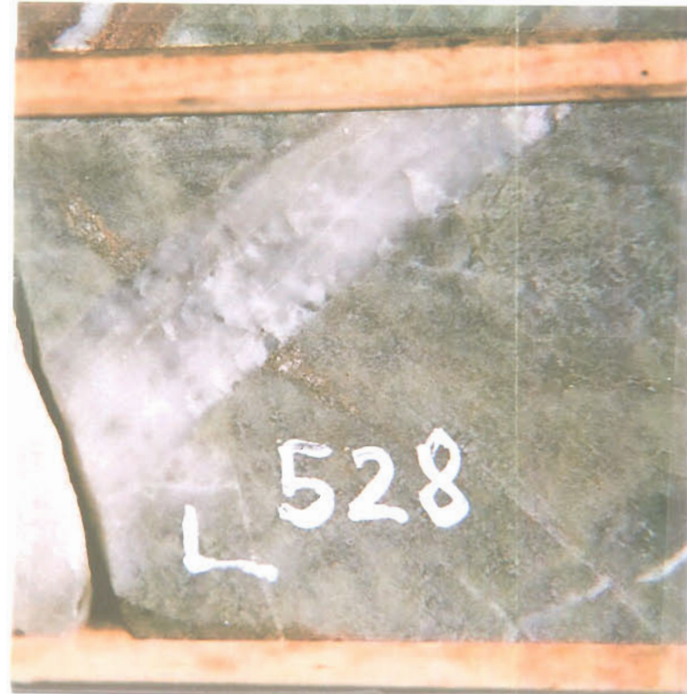
Pyrite veins crosscut by quartz tension gashes (51529, 51528).
