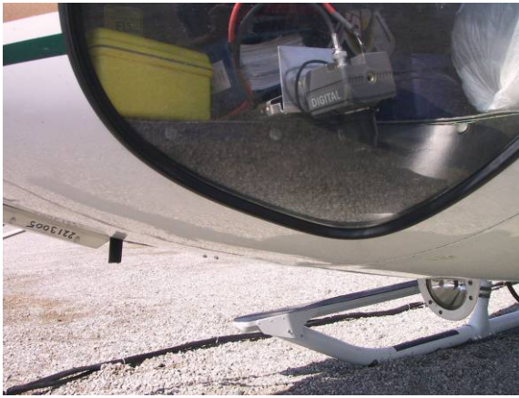
Figure 7. Digital video camera typical mounting location
