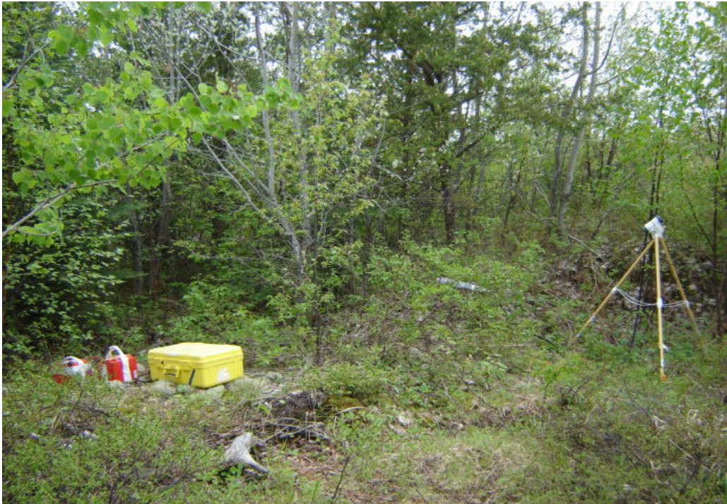
Figure 5: CF1 Magnetic Base Station Set-up
