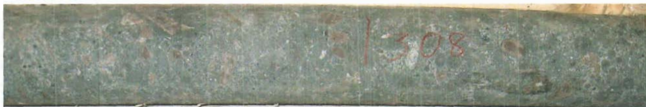
Image 10: Photograph of phase three volcaniclastic breccia from TD-08-10 illustrating the lapilli-rich nature of the unit (and segregation textures) and dark red, iron-altered clasts.
