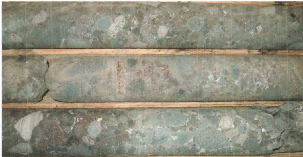
Image 9: Photograph of phase two (TD-08-10) illustrating the matrix-supported texture and iron alteration of the subangular clasts.
