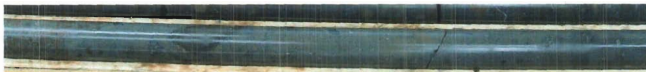
Image 3: Photograph of fine-grained, matrix-supported (<20% clasts), volcanoclastic dyke crosscutting both the early phases of volcanoclastic breccia (similar to phase four in TD-08-08).
