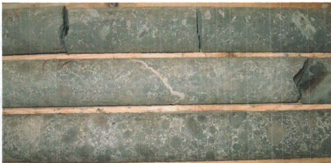
Image 6: Photograph of the lapilli-rich, segregation-textured volcanoclastic breccia with rounded juvenile lapilli surrounded by calcite (phase three).
