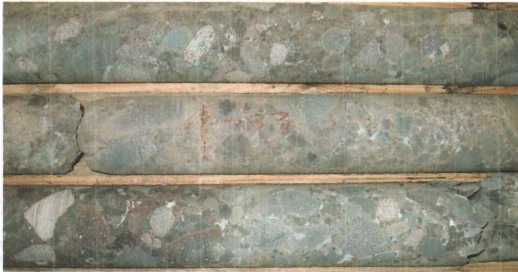
Image 8: Photograph of clast-supported volcanoclastic breccia (phase one) illustrating interstitial calcite, dark red (iron-altered) lapilli and rounded clasts.
