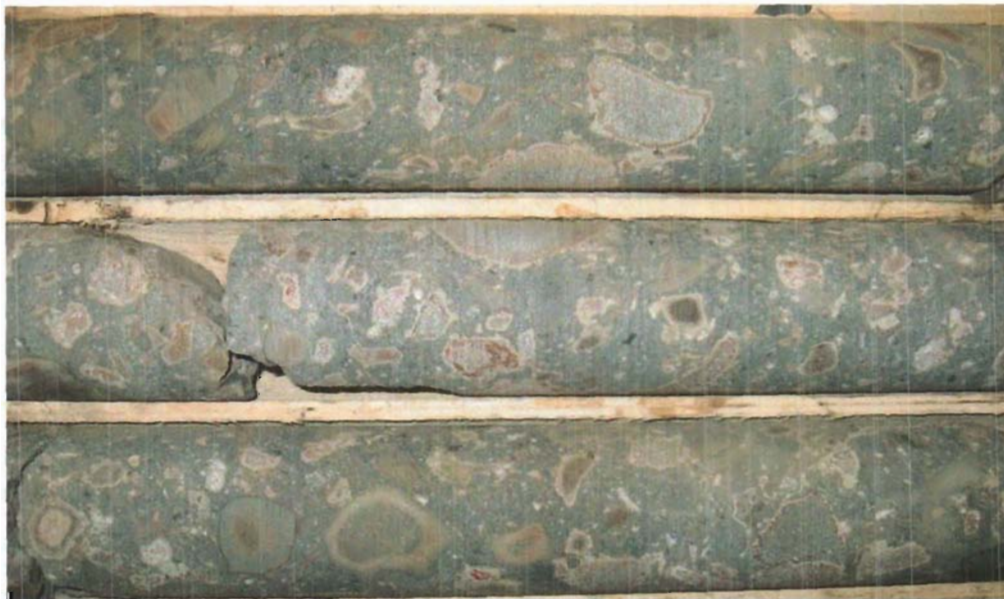
Image 5: Photograph of the matrix-supported volcanoclastic breccia with subangular, iron-altered clasts set in a dark grey-green matrix (phase two).
