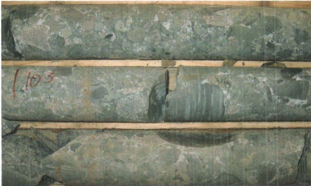
Image 4: Photograph of clast-supported (40-90%) heterolithic breccia with white interstitial calcite and rounded to subangular clasts (phase one).
