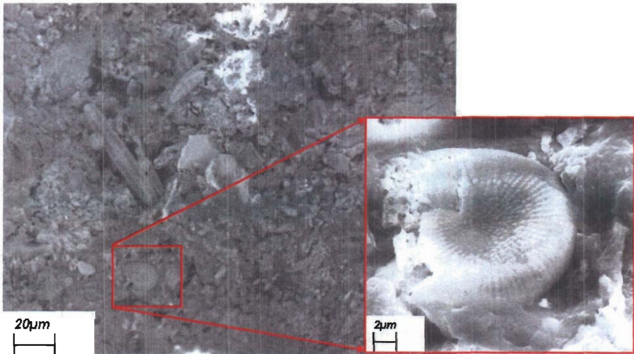
Figure 4: BSE image of grain 3413-1 with a secondary electron image box-out of a selected diatom.
