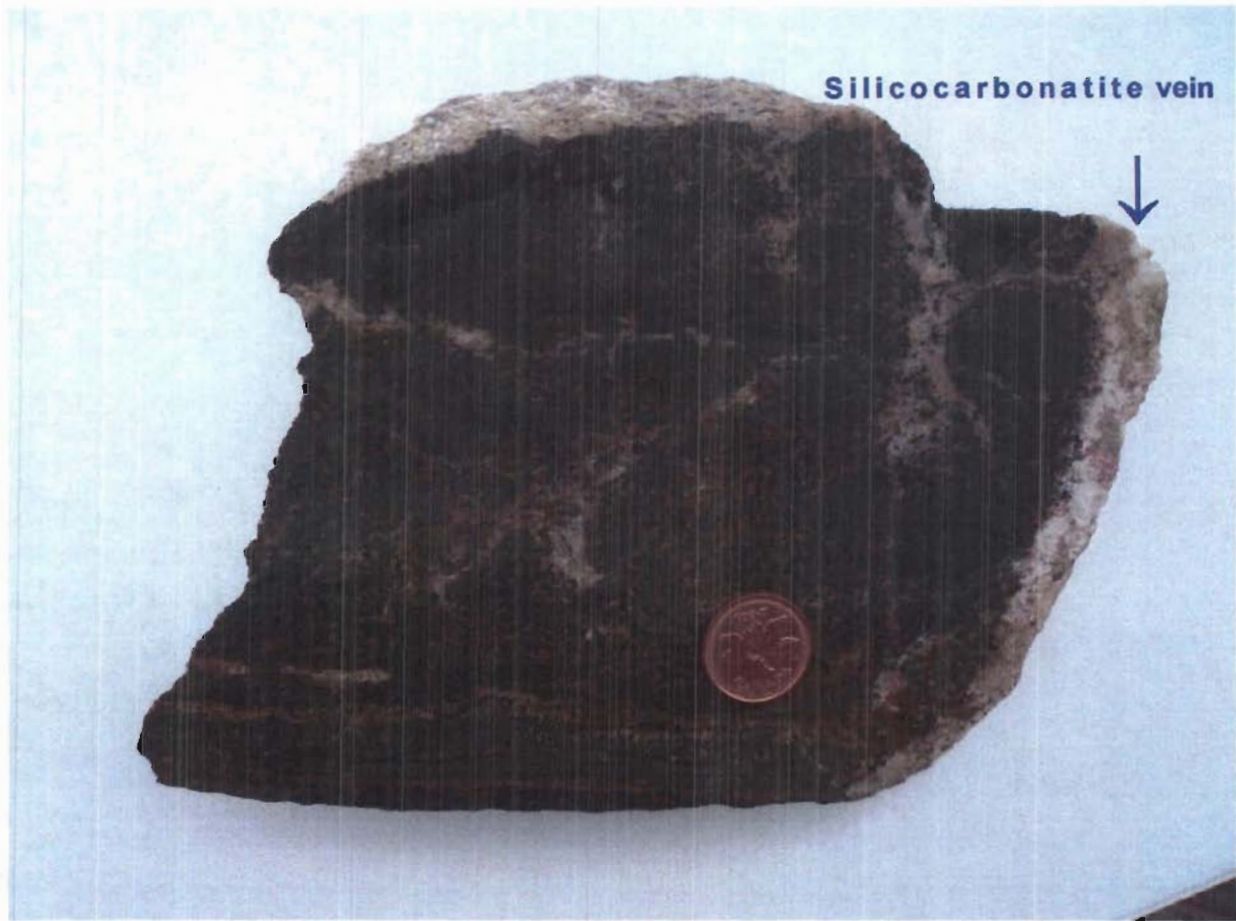
Photo 5. Part of a silicocarbonatite vein (arrow) and related veins and patches in a deep green to black ijolite host-rock from locality 3429. The deep green, medium- to coarse-grained mineral is possibly aegerine-augite (as above coin) that may have evolved via fenitization of the foliated ijolite host. The light pink phase is likely natrolite.
