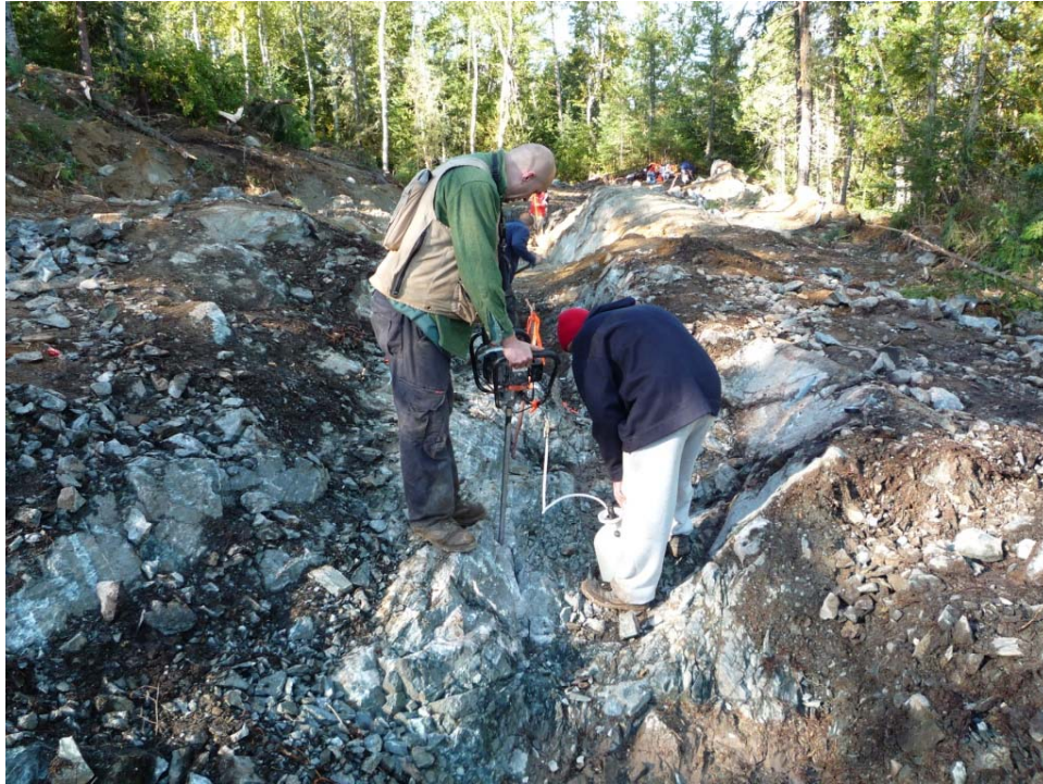
Figure 8: Pressuring-up portable core drill in preparation for coring at the Flint Rock occurrence.
