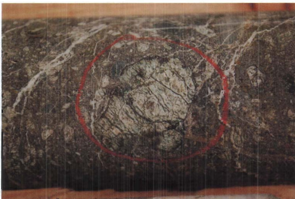
Figure 4f: Mantle xenolith composed by olivine and \pm Cr-diopside in hole 08-MF2-01
