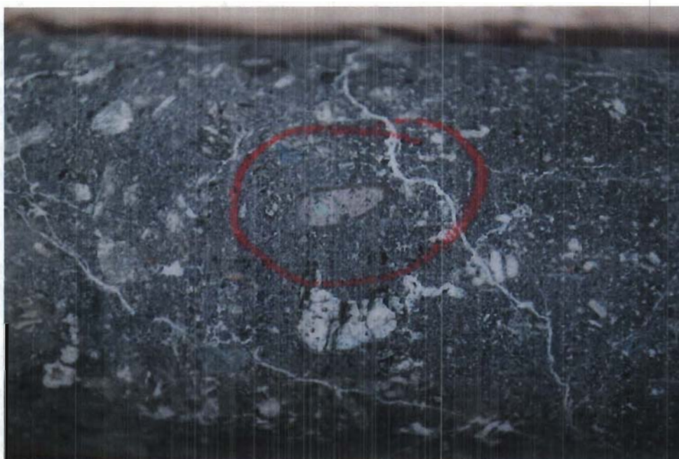
Figure 4b: Xenolith composed with purple garnet and \pm Cr-diopside with kelyphitic rim in hole 08-MF2-01
