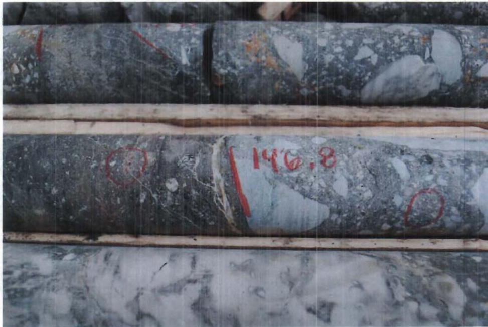
Figure 4c: Young kimberlite (dark grey brown) cutting older kimberlite (medium grey, rich in limestone xenoliths) with sharp contact at 146.8m in hole 08-MF2-01
