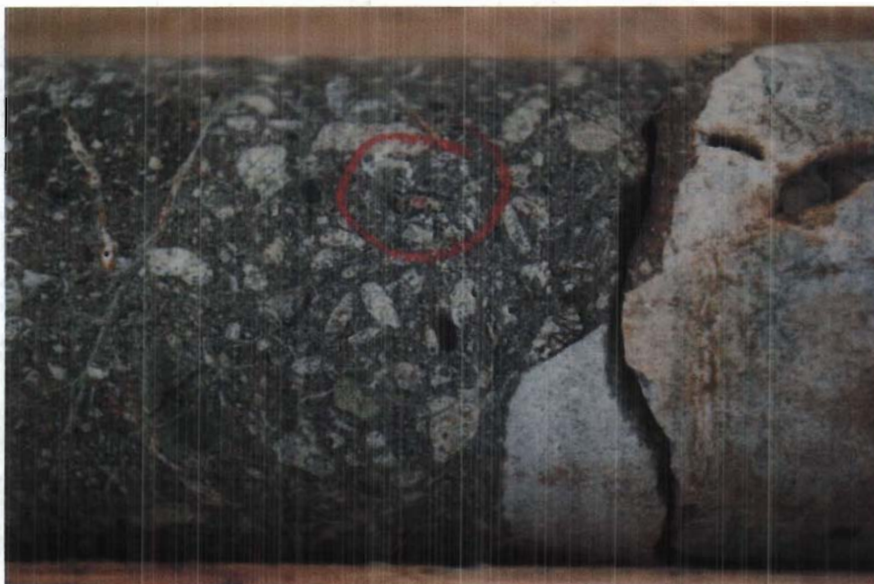
Figure 4e: Dark grey autholith and dark pink garnet with kelyphitic rim in hole 08-MF2-01
