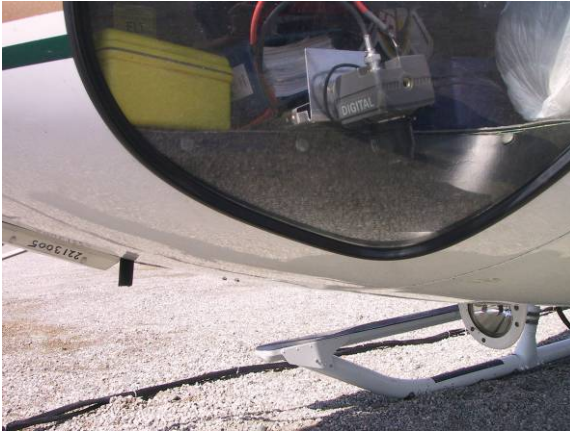
Figure 7. Digital video camera typical mounting location.
