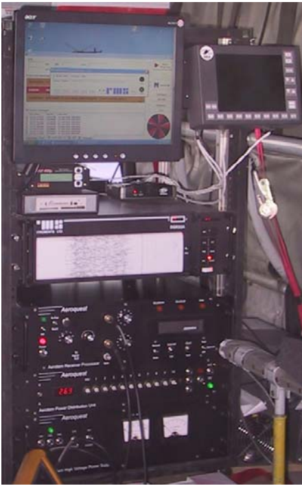
Figure 6. AeroTEM IV Instrument Rack., including AeroDAS and RMS DGR-33 systems, AeroTEM power supply, data acquisition computer and AG-NAV2 navigation system.
