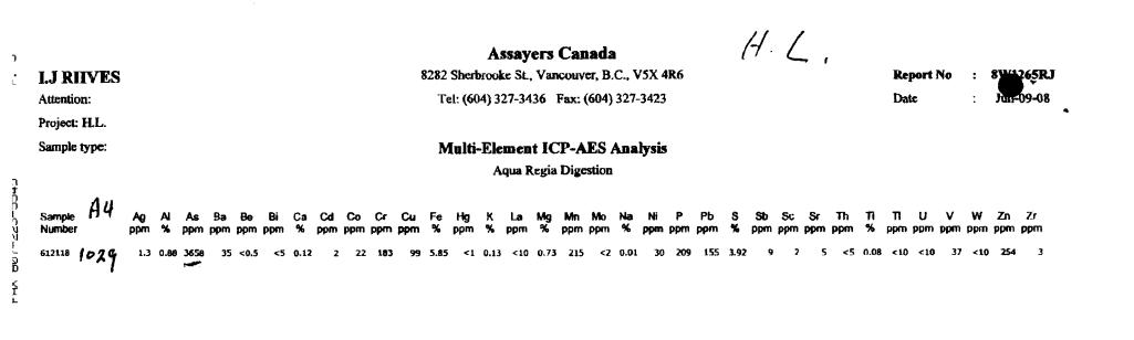
A .5 gm sample is digested with 5 ml 3:1 HCI/HNO3 at 95°C for 2 hours and diluted to 25ml.
