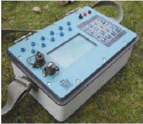
ELREC Pro unit with its graphic LCD screen
