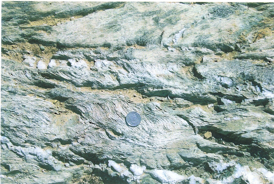
Photo 16. A location of complex shearing with two dextral and one sinistral shear zones. See text for details. Station 46.
