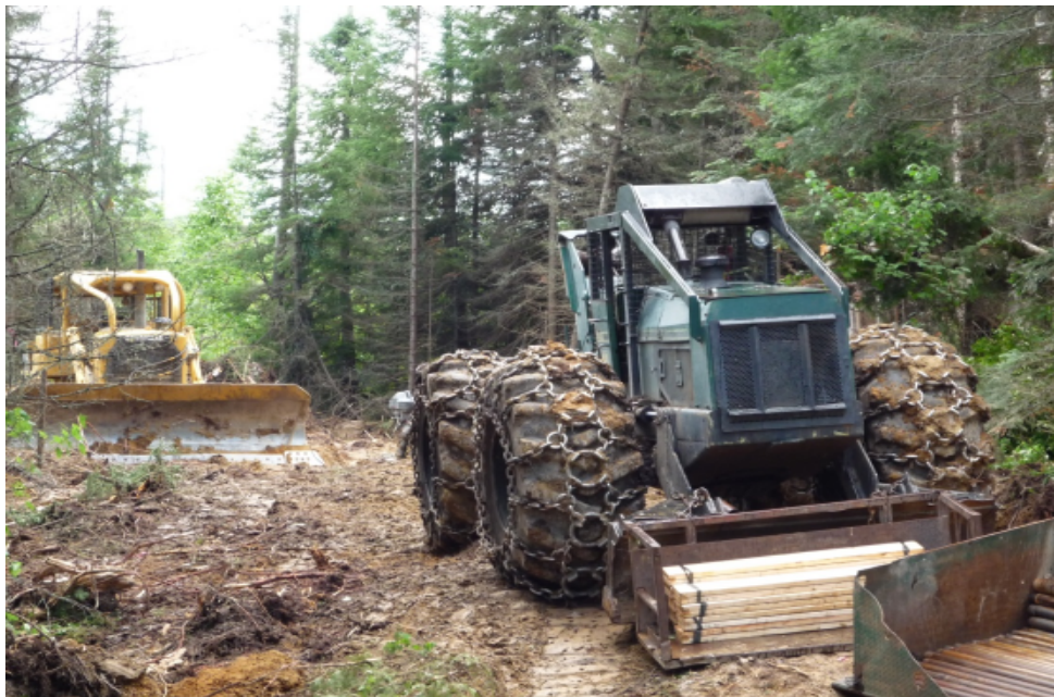
Figure 4: C7 Timberjack skidder in the foreground hauling core boxes, with a D7 Caterpillar dozer in the background.
