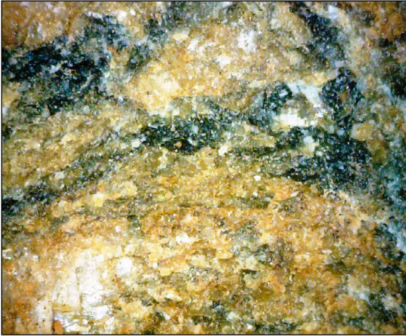
Figure 5 X 400 views of inclusions and septas in quartz vein (claim 4202099)
