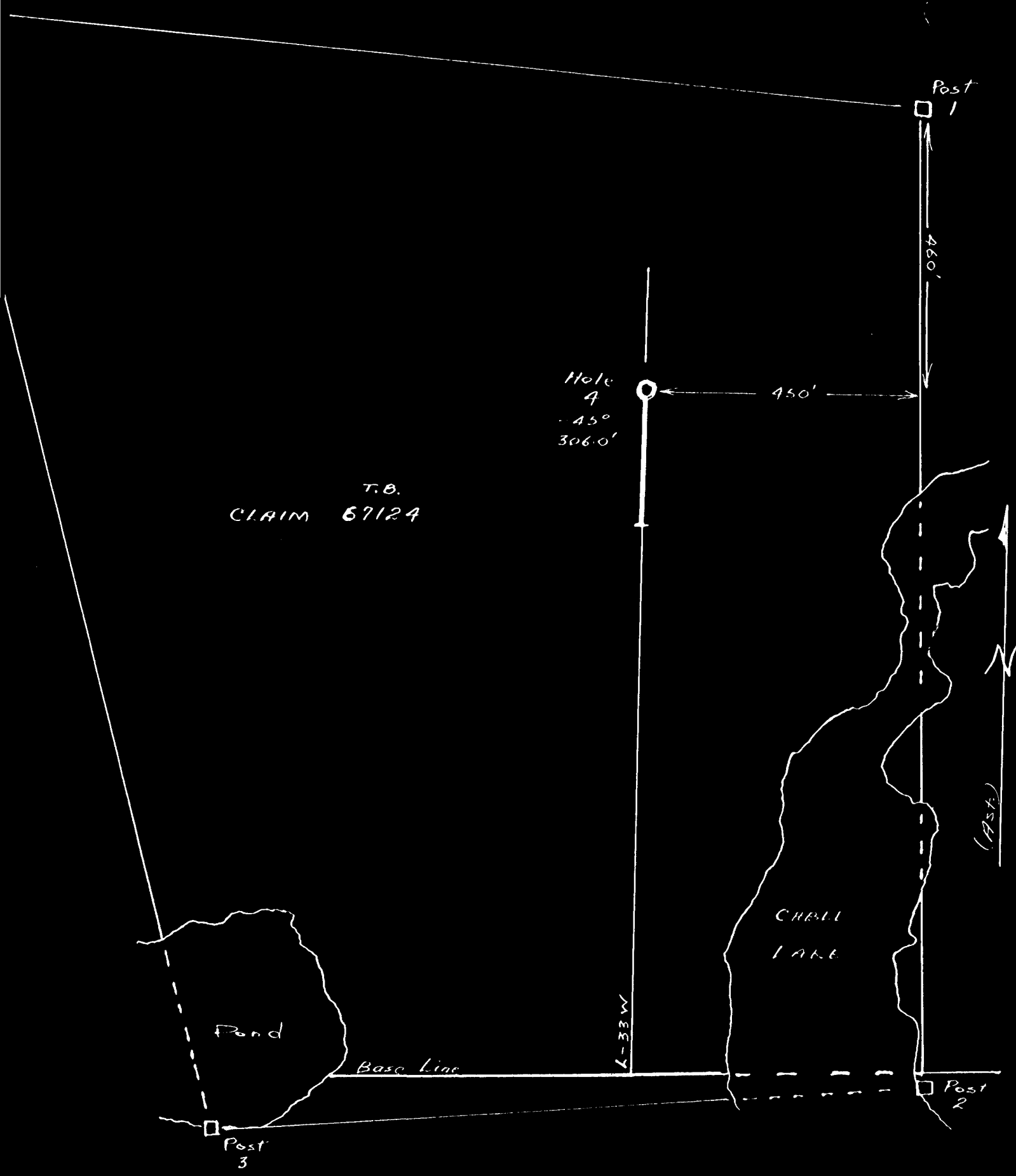
Sketch showing location of HOLE 4 in relation to corner posts Scale 1 inch = 200 feet
