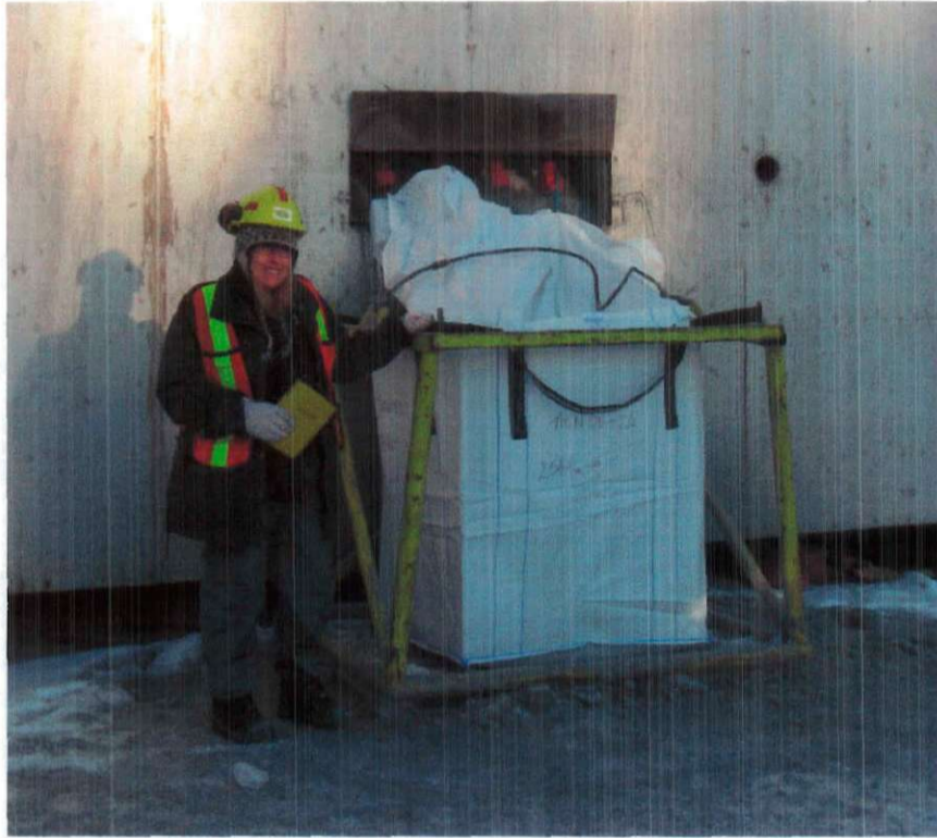
Figure 8: Fine fraction (<0.5mm) that passed through the shaking table being collected in sample bags outside the drill shack.
