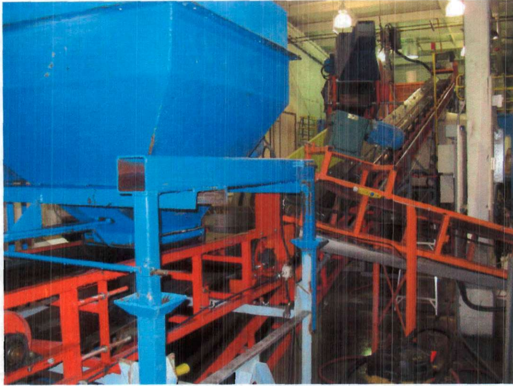
Figure 10: The conveyor feed system for the DMS at Microlithics Laboratory, Thunder Bay.
