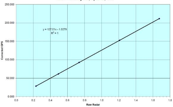
Terraquest LTD Radar Altimeter Calibration 20/04/2010
