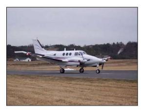
The Beech King Air 90 is an ideal platform for carrying out an airborne geophysical survey in these demanding environmental conditions. It is IFR equipped with twin PT6-20 turbines that will ensure reliability at both high ferry speed and slow survey speed. It is equipped with the long-range tanks capable of carrying approximately six hours of fuel.
