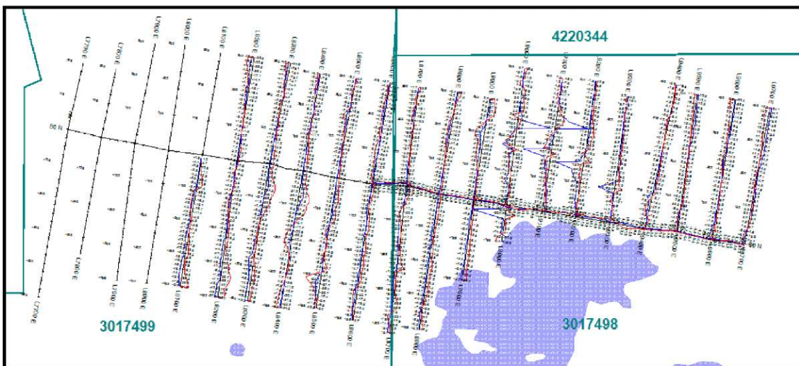
Figure 2. VLF offset profiles, 24.0 kHz
