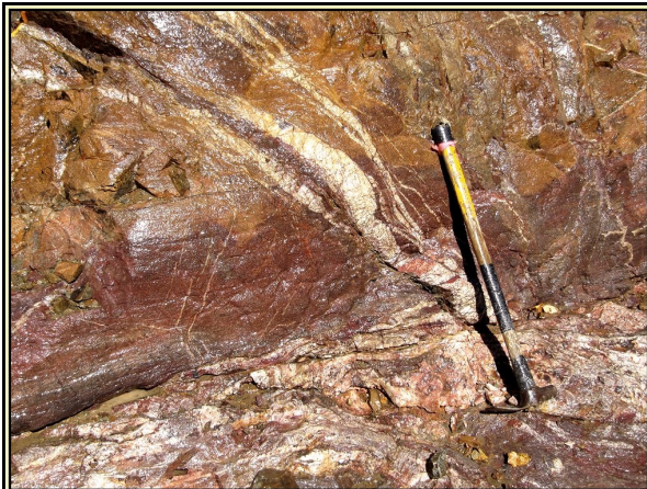
Figure 8: Cu-Mo Zone, showing multiple sets of quartz stringers and hematitic alteration
