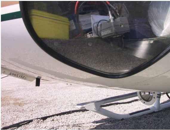
Figure 7. Digital video camera typical mounting location
