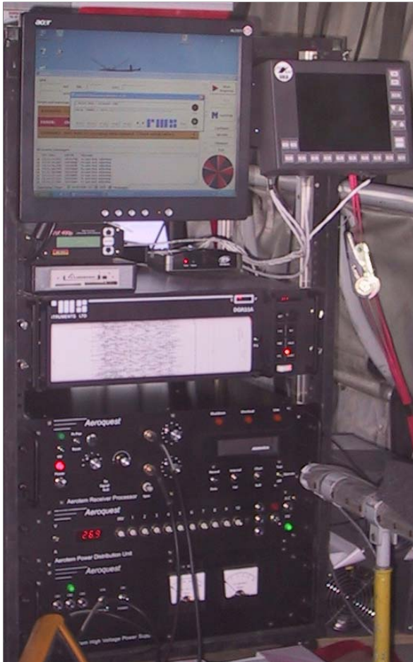
Figure 6. AeroTEM III Instrument Rack
