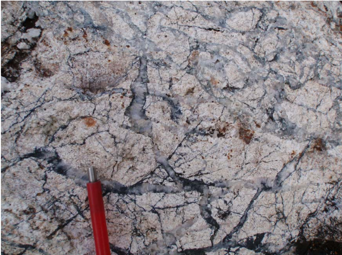
Plate 3: Quartz-tourmaline stockwork veins in porphyry.
