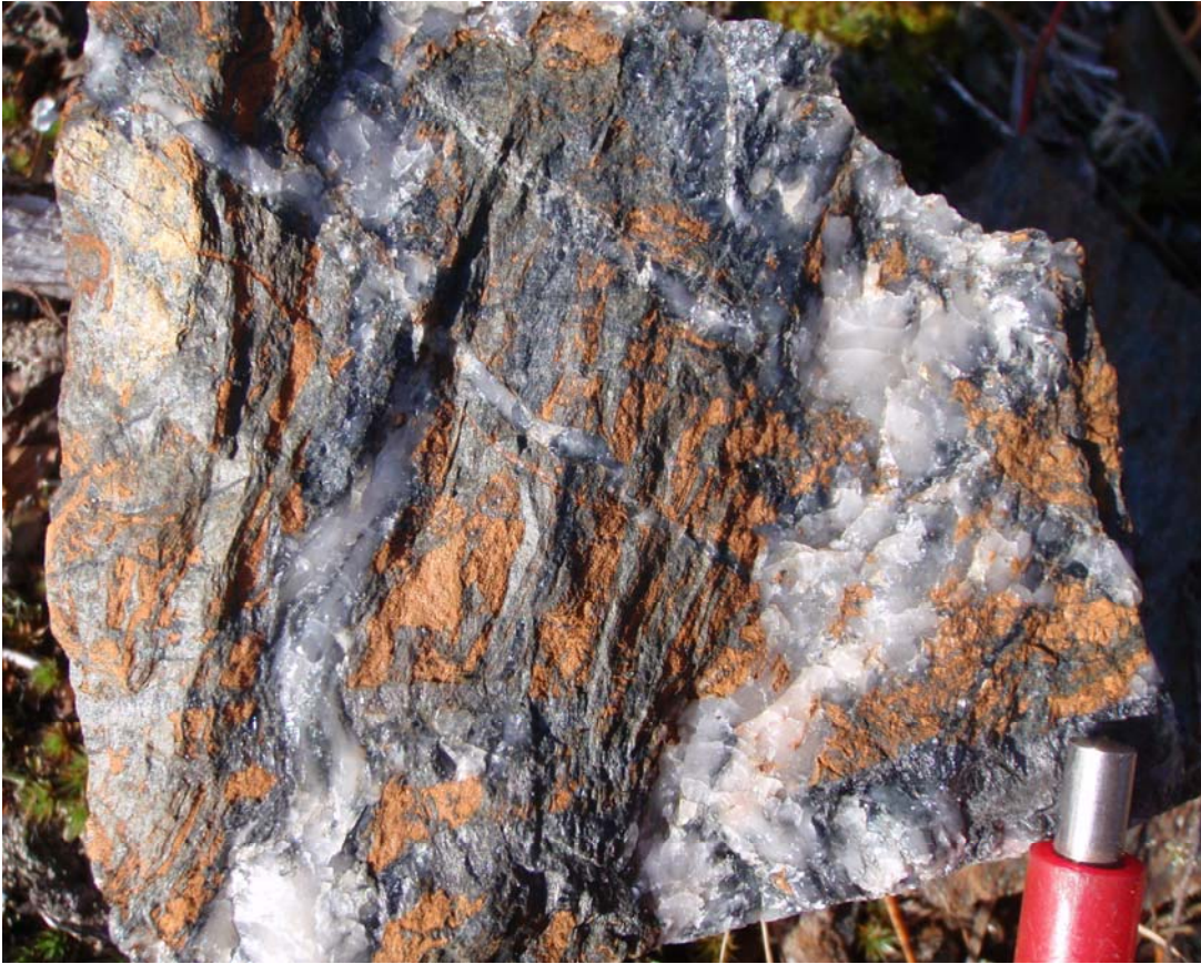
Plate 5: Multi-stage quartz veins cutting strong iron carbonate alteration.
