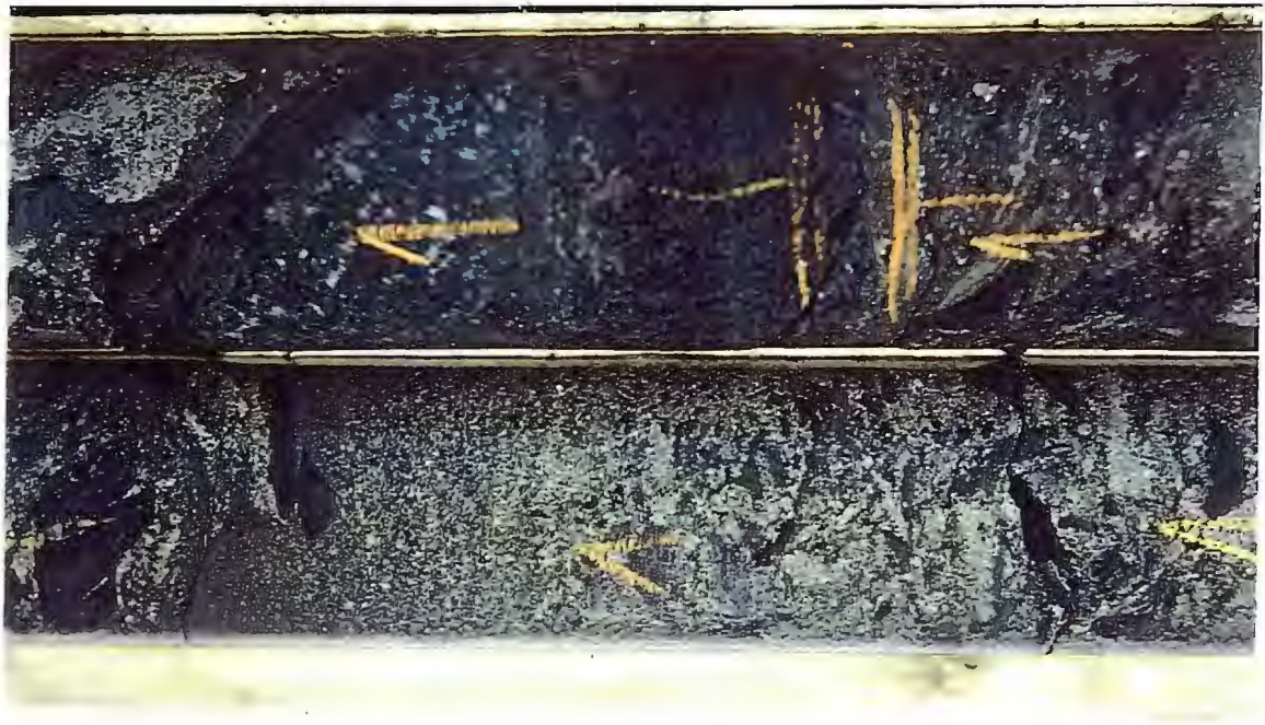
Graded magmatic bed of chalcopyrite in ultramafic magma at Hollinger Copper
