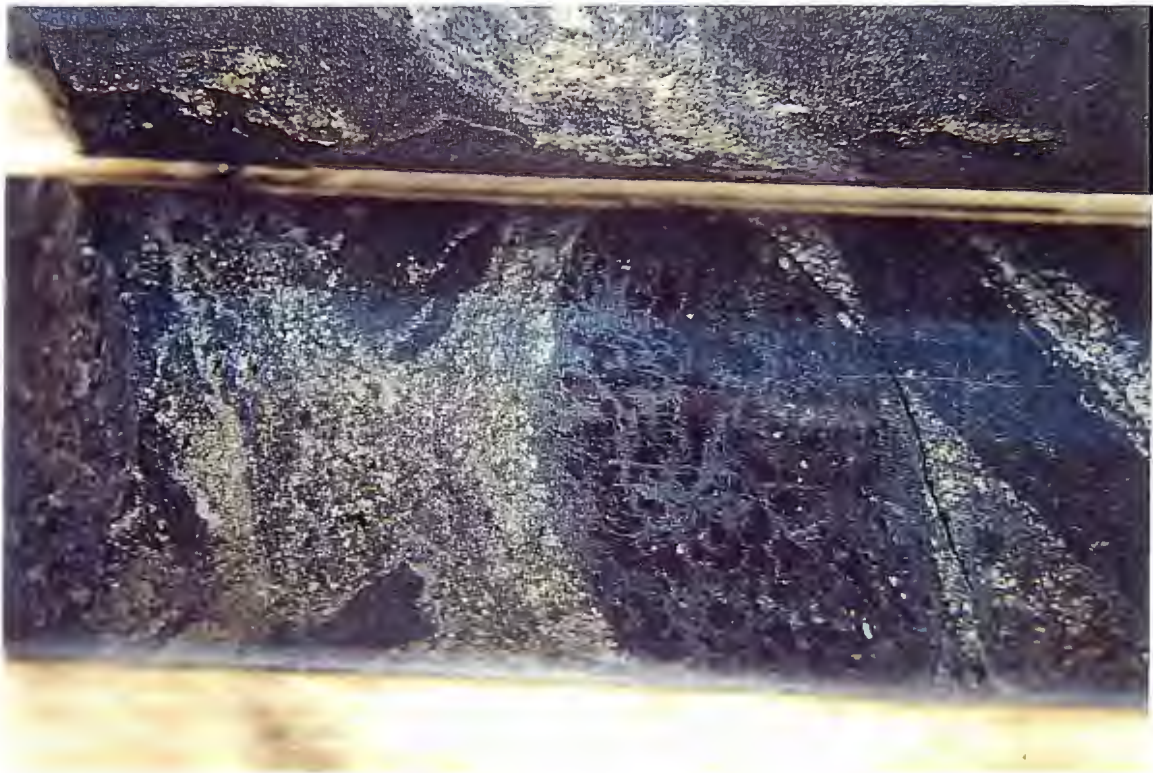
Serpentinite wallrock fragments in chalcopyrite slush at base of next bed just above
