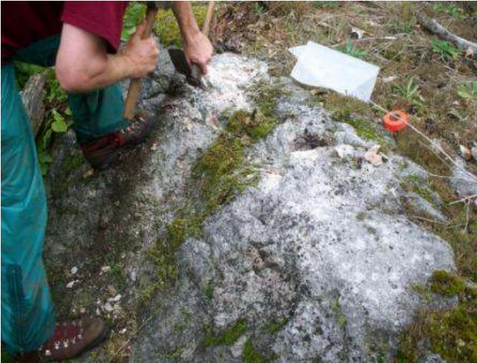
Raglan Twp. Claim # 3006548 (Melkior option) Sample: HN-23, coarse grained k-spar and qtz with minor amphibole.
