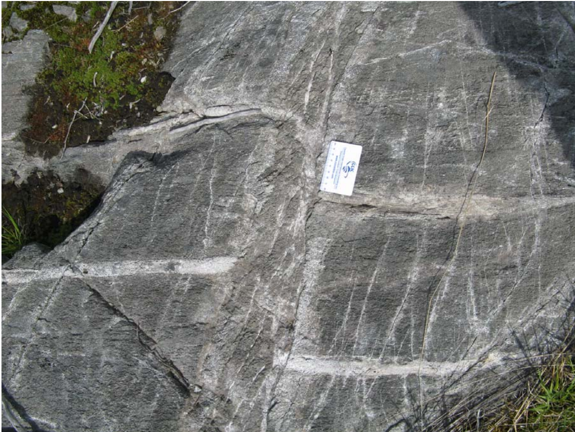
Figure 9-3. Chloritic biotite schist with 13 cm wide fault zone, 352°/85, 16cm dextral displacement of feldspar vein. (8+85W, 4+30S, UTM 527879E, 5511200N, zone 15, NAD83).
