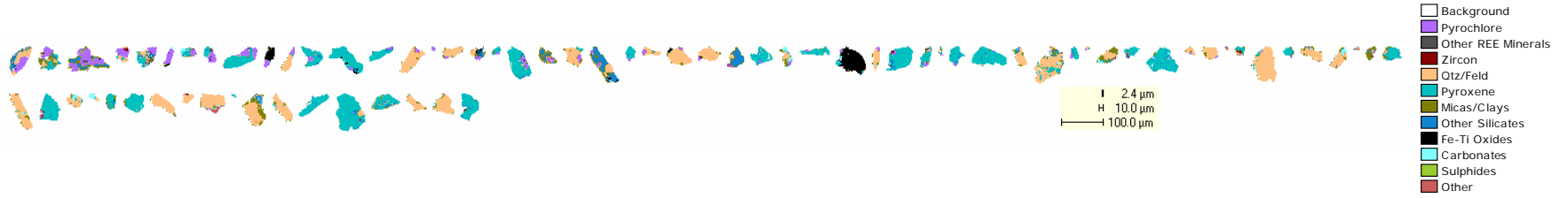
Figure 27: Image Grid Displaying Complex Pyrochlore Particles for the -75/+25 µm Fraction
