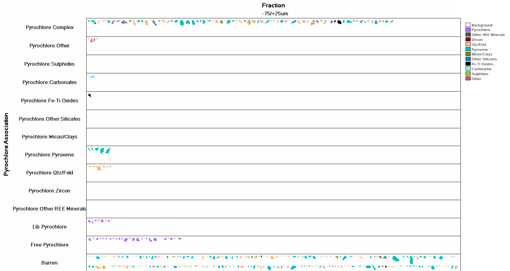
Figure 26: Image Grid Displaying Pyrochlore Liberation and Association for the -75/+25 µm Fraction
