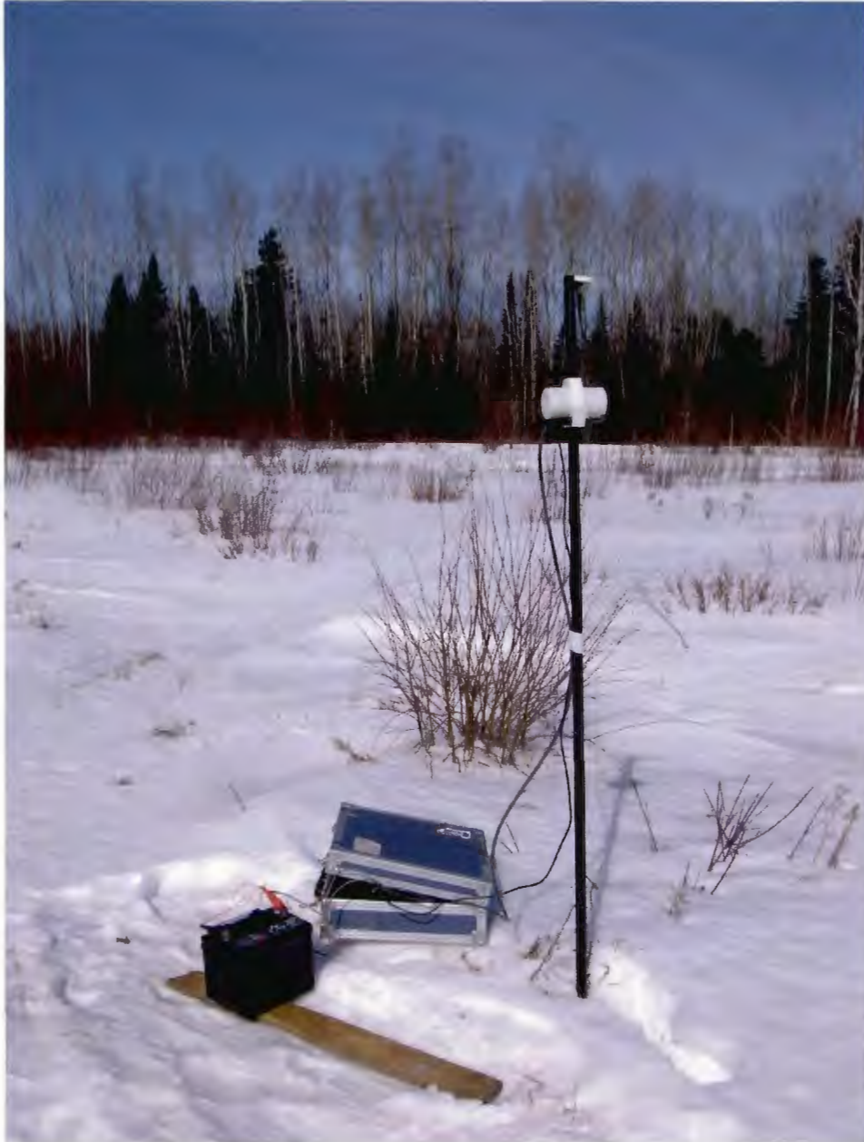
Figure 5: Example of a GEM Base Station Setup
