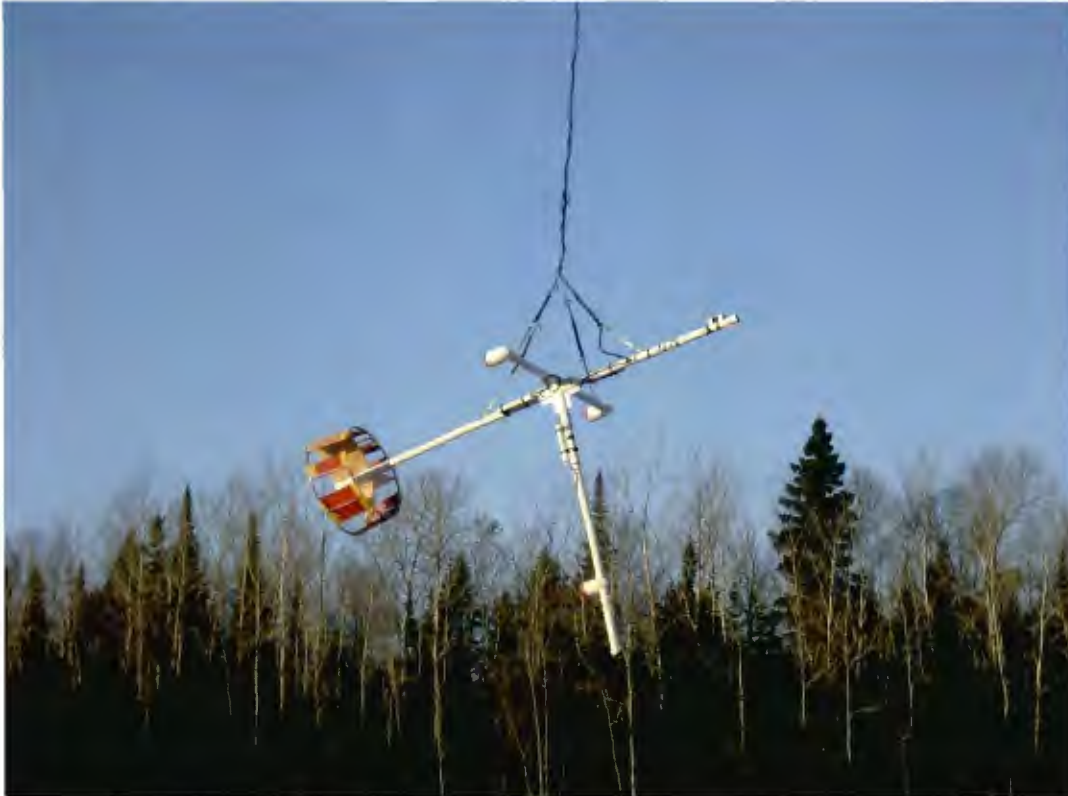
Figure 2: Fugro Airborne Surveys Tri-Axial Mounted Magnetic Gradiometer bird
