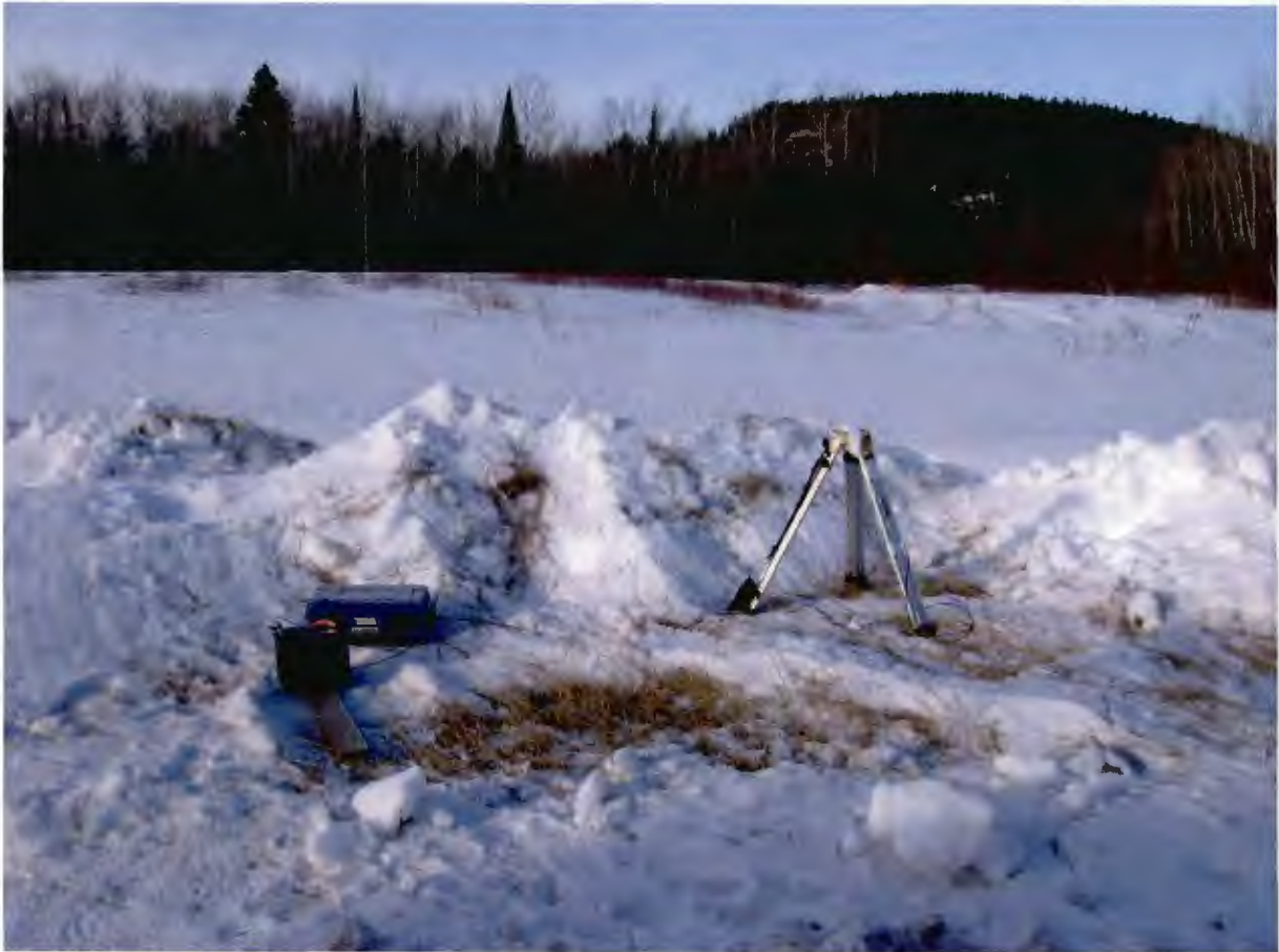
Figure 6: Example of a GPS Base Station Setup
