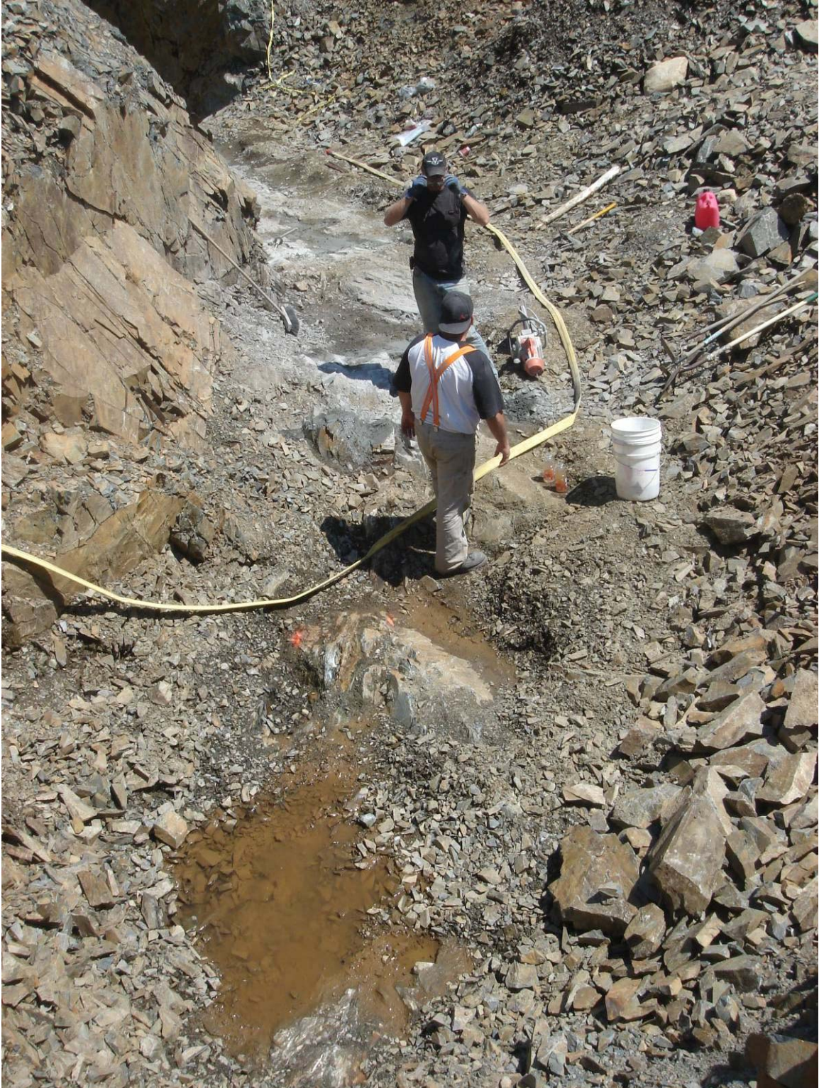
Plate 2. J.Burt and D.Ranville channel sampling Triggs Trench Sampling of the trench with work half completed is illustrated above.
