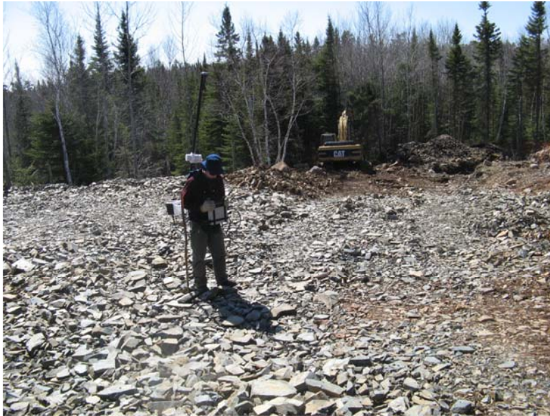
Figure 4. Photograph of the Gem Systems GSM-19mag/vlf/cdgps system at 12.5m S on Line 1050W.
