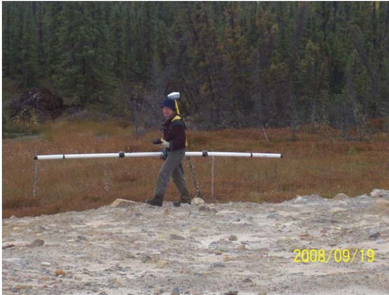
Figure 6. The EM-31MK2 and DGPS system are shown in operation above.
